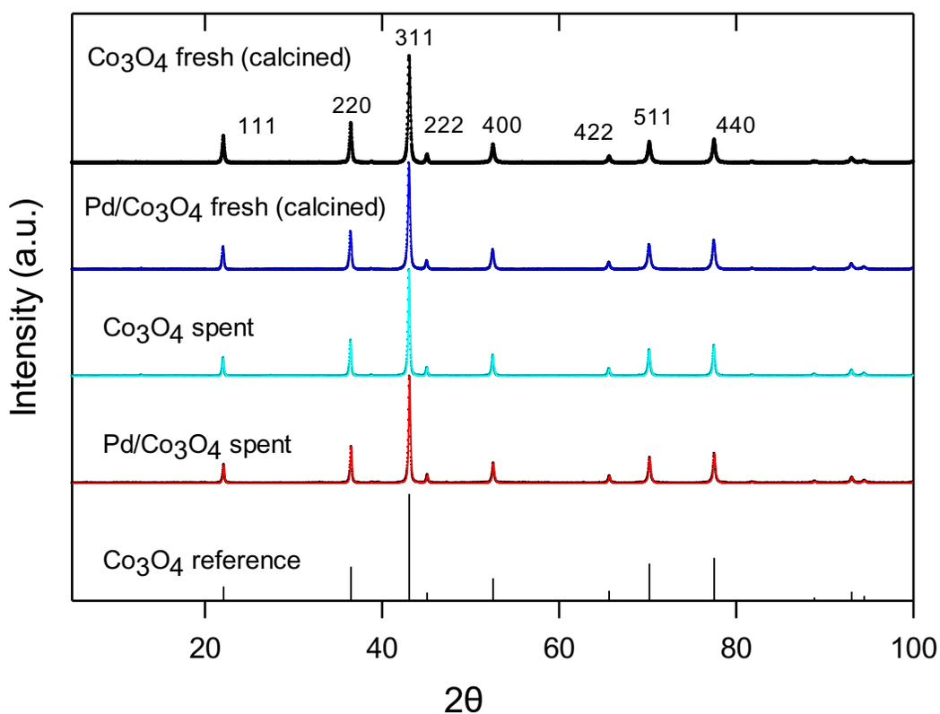
Figure 3.1 XRD profiles of the fresh and spent catalysts.
