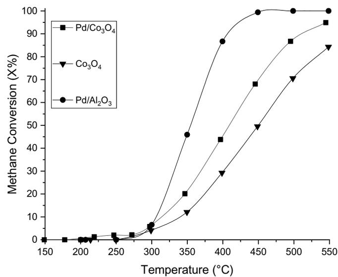
Figure 4.10 Methane combustion activity of the prereduced catalysts (300 °C, in H<sub>2</sub>) in the wet feed. 0.3 g catalyst loading, with 0.3 wt.% Pd in each of Co<sub>3</sub>O<sub>4</sub> and Al<sub>2</sub>O<sub>3</sub>. Pd dispersion is 12% in Pd/Co<sub>3</sub>O<sub>4</sub> and 40% in Pd/Al<sub>2</sub>O<sub>3</sub>.
