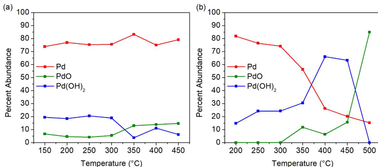
Figure 4.9 Pd speciation from *in situ* XAS during wet methane combustion starting with the reduced catalysts: (a) Pd/Co<sub>3</sub>O<sub>4</sub> with Pd dispersion of 12% and (b) Pd/Al<sub>2</sub>O<sub>3</sub> with Pd dispersion of 40%. reprinted from [30] with permission, copyright John Wiley and Sons, 2019.
