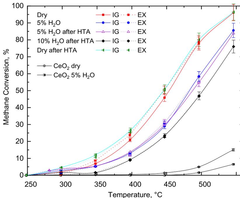
Figure 5.4 Ignition (IG) and extinction (EX) curves on  $\text{Co}_3\text{O}_4/\text{CeO}_2$  catalyst in the dry and wet feeds before and after 68 hours of hydrothermal ageing (HTA) with 5% water.
