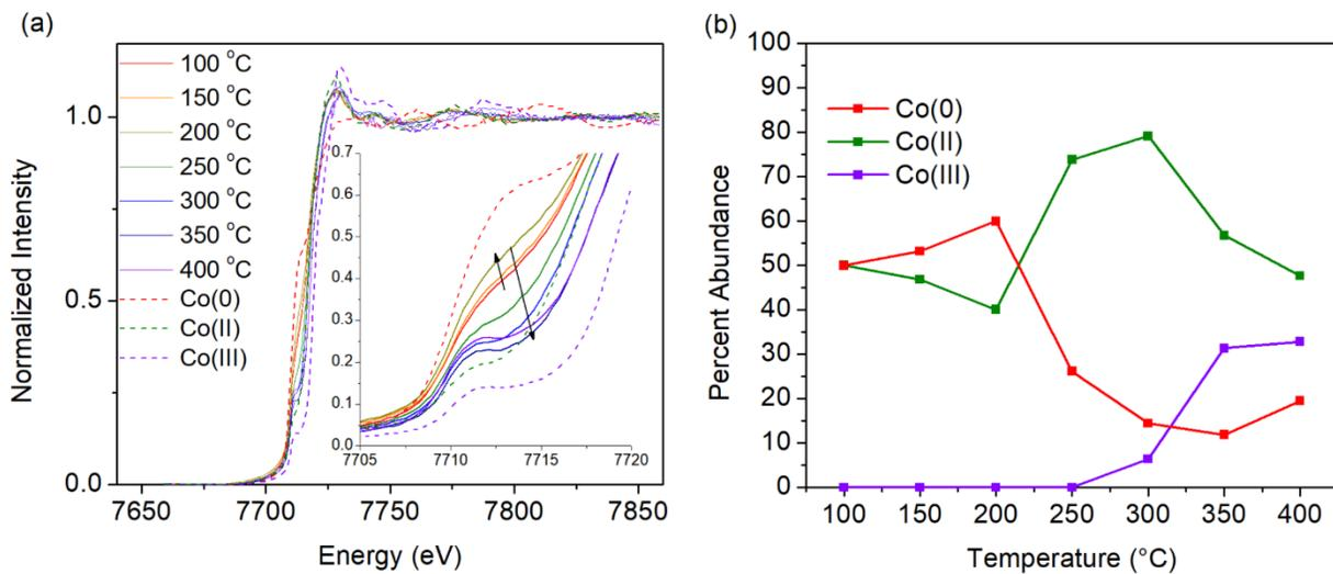
Figure 4.7 . Co K edge XAS spectra of Pd/CoO<sub>x</sub> a) during in situ wet combustion and b) with linear combination fitting.
