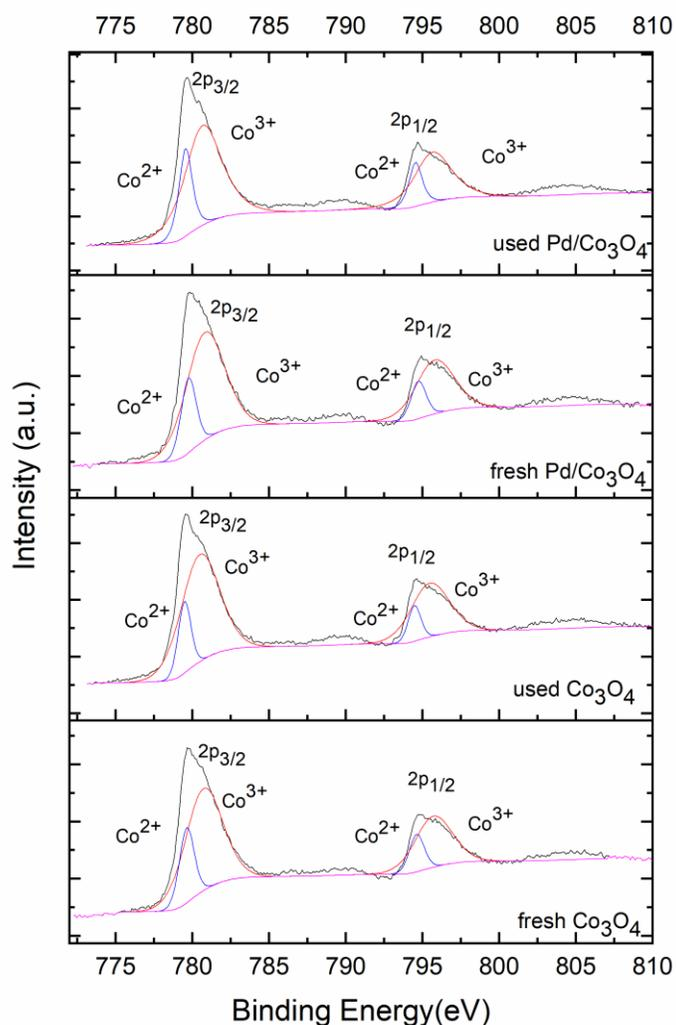
Figure 4.1 XPS profiles of Co<sub>3</sub>O<sub>4</sub> and Pd/Co<sub>3</sub>O<sub>4</sub> catalysts: fresh (calcined) and used in wet methane combustion for one week on stream. The quantitative analysis can be found in Table 4-4-1 in the Supporting Information.
