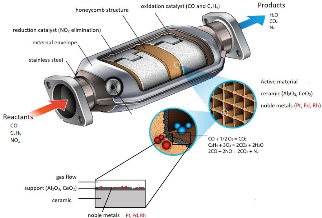
Figure 1.1 . Schematic of catalytic converter. Adapted with permission from [7].
