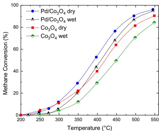
Figure 4.4 Methane combustion activity of the reduced catalysts in the dry and wet feed. 600 ppmv CH<sub>4</sub>, 1 mol.% H<sub>2</sub>O, 0.3 g of catalysts, Pd dispersion is 12%.
