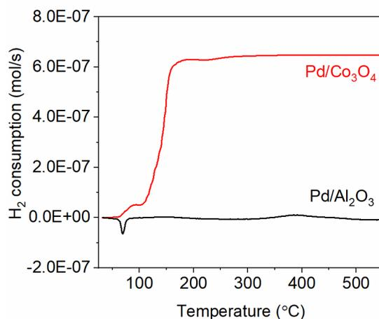
Figure 4.6 TPR in H<sub>2</sub> at 10 °C/min heating rate (0.5 g of each sample). A Pd/Al<sub>2</sub>O<sub>3</sub> catalyst is shown for comparison to demonstrate that Co reduction is the primary cause of H<sub>2</sub> consumption, presumably by spillover of activated hydrogen from β-Hydride of Pd. Reproduced with permission from [109], copyright 2019, Elsevier.
