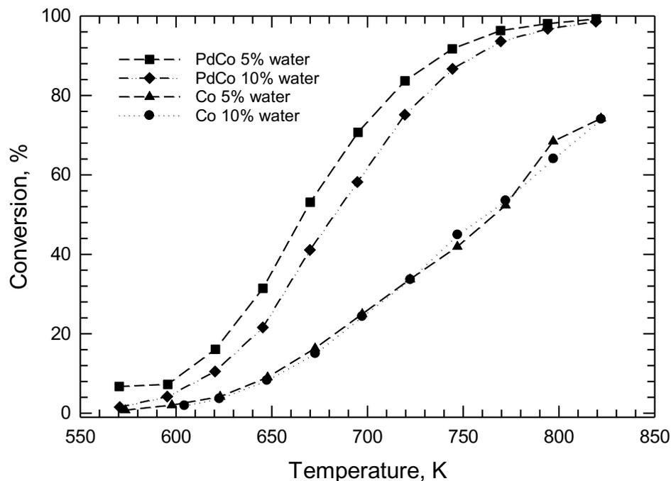
Figure 3.4 Ignition curves in catalytic methane combustion of the wet lean feed, 0.6 g catalyst ( $\text{Co}_3\text{O}_4$  or  $\text{Pd}/\text{Co}_3\text{O}_4$ , 0.27 wt.% Pd), 210 mL<sub>STP</sub>/min, 5000 ppm  $\text{CH}_4$ , 19.5 vol. %  $\text{O}_2$ , GHSV = 21,000 L<sub>(STP)</sub>/(kg<sub>cat</sub>·h). The data are for Trial 2 (T2).
