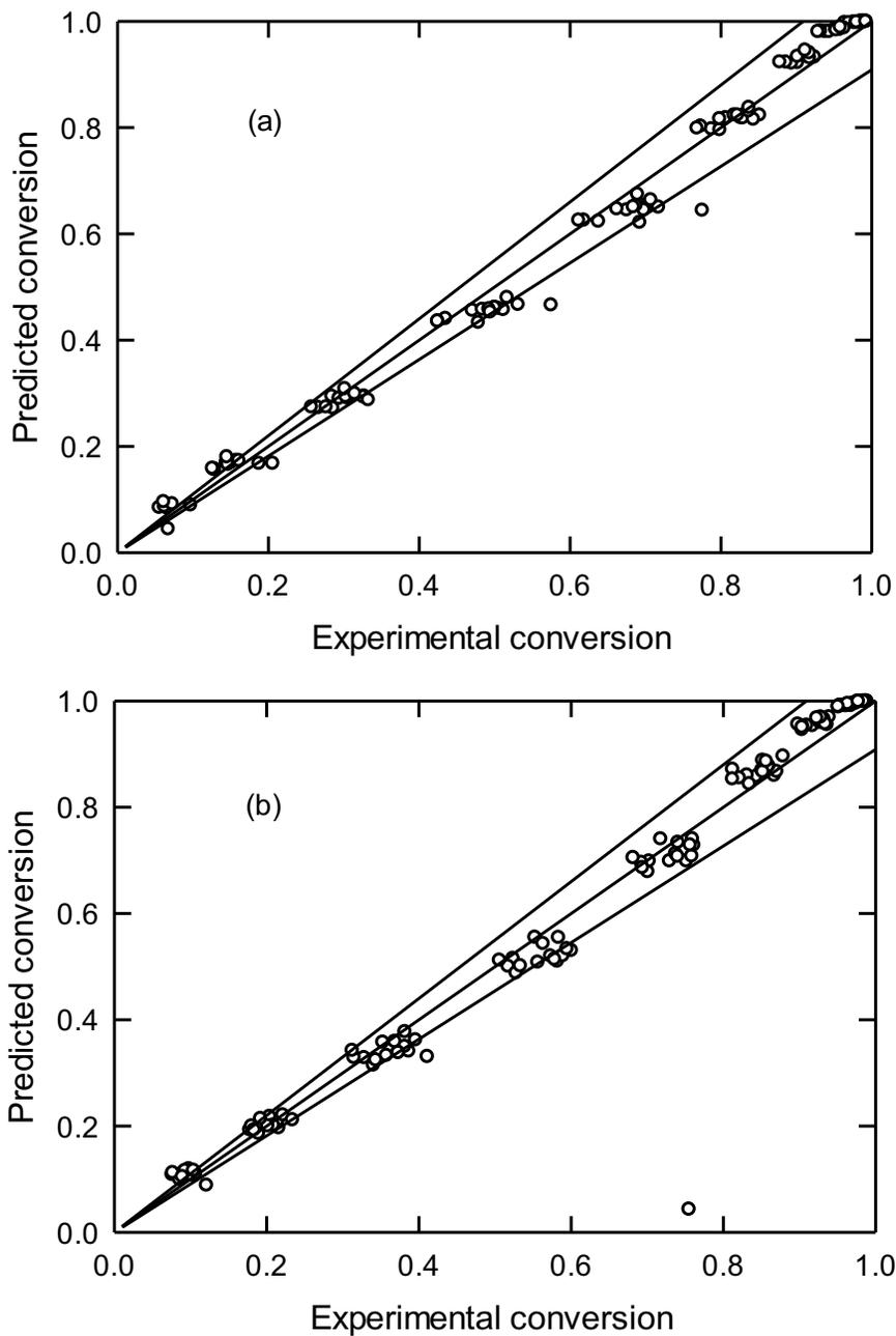
Figure 3.11 . Parity plots with plus and minus 10 % error range for the Pd/Co<sub>3</sub>O<sub>4</sub> catalyst with the conversions predicted using 1<sup>st</sup> order to methane and Arrhenius law parameters from Table 1. (a) 5% water and (b) 10 % water. Reaction conditions are the same as given in Figure 3.8.
