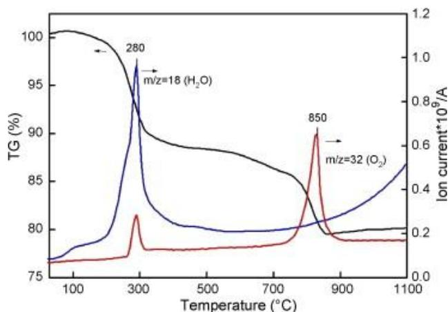
Figure 1.6 Thermogravimetric analysis of the outlet gases from the decomposition of CoO(OH) by TG-MS H<sub>2</sub>O (blue) and O<sub>2</sub> (red). Reprinted from [62] with permission from Elsevier copyright 2008.
