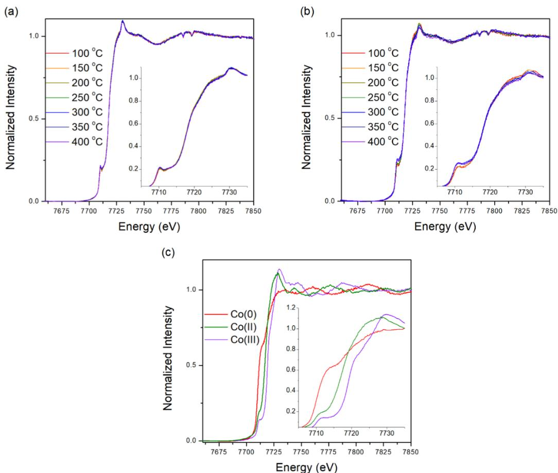
Figure 4.3 Co K edge *in situ* XAS data of the Pd-free cobalt oxide catalyst under a) dry, b) wet methane combustion conditions and c) cobalt standards.
