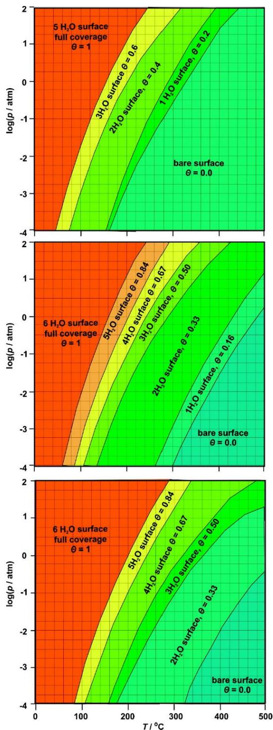
Figure 1.3 Two-dimensional diagrams of water coverage as a function of temperature and partial pressure of water for (a, top panel) (100), (b, middle panel) (110), and (c, bottom panel) (111) planes of cobalt spinel. Reprinted from [61] with permission from American Chemical Society copyright 2010.
