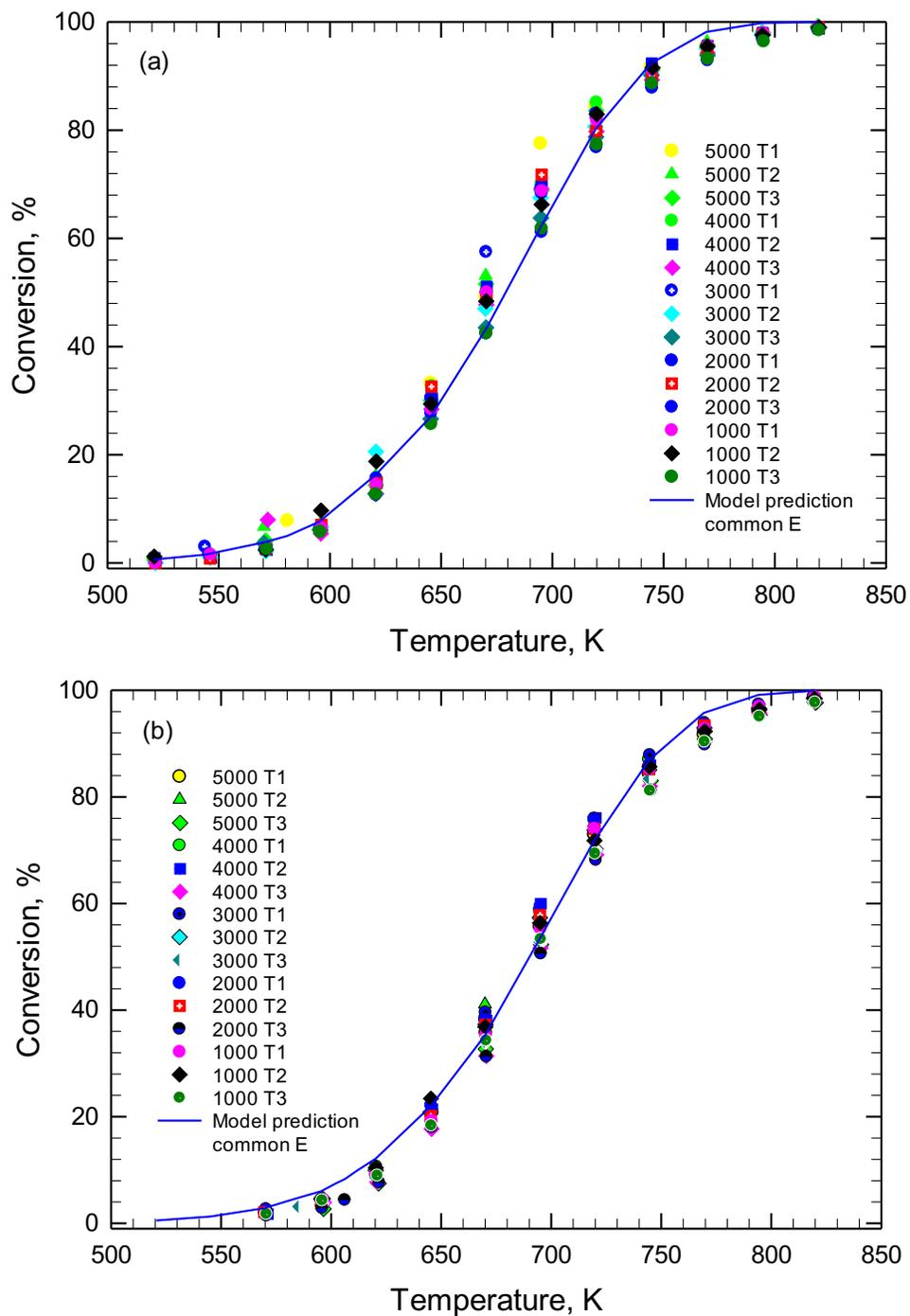
Figure 3.6 Ignition curves for Pd/Co<sub>3</sub>O<sub>4</sub> (Pd 0.27 wt. %) catalyst for three trials (T1-T3) at different CH<sub>4</sub> concentrations (ppmv) at (a) 5 vol. % H<sub>2</sub>O (a) and (b) 10 vol. % H<sub>2</sub>O in the feed. Reaction conditions are the same as for the Co<sub>3</sub>O<sub>4</sub> catalyst (Fig. 2). The model is based on the parameters in Table 3-2 with a common activation energy of 90.7 kJ/mol.
