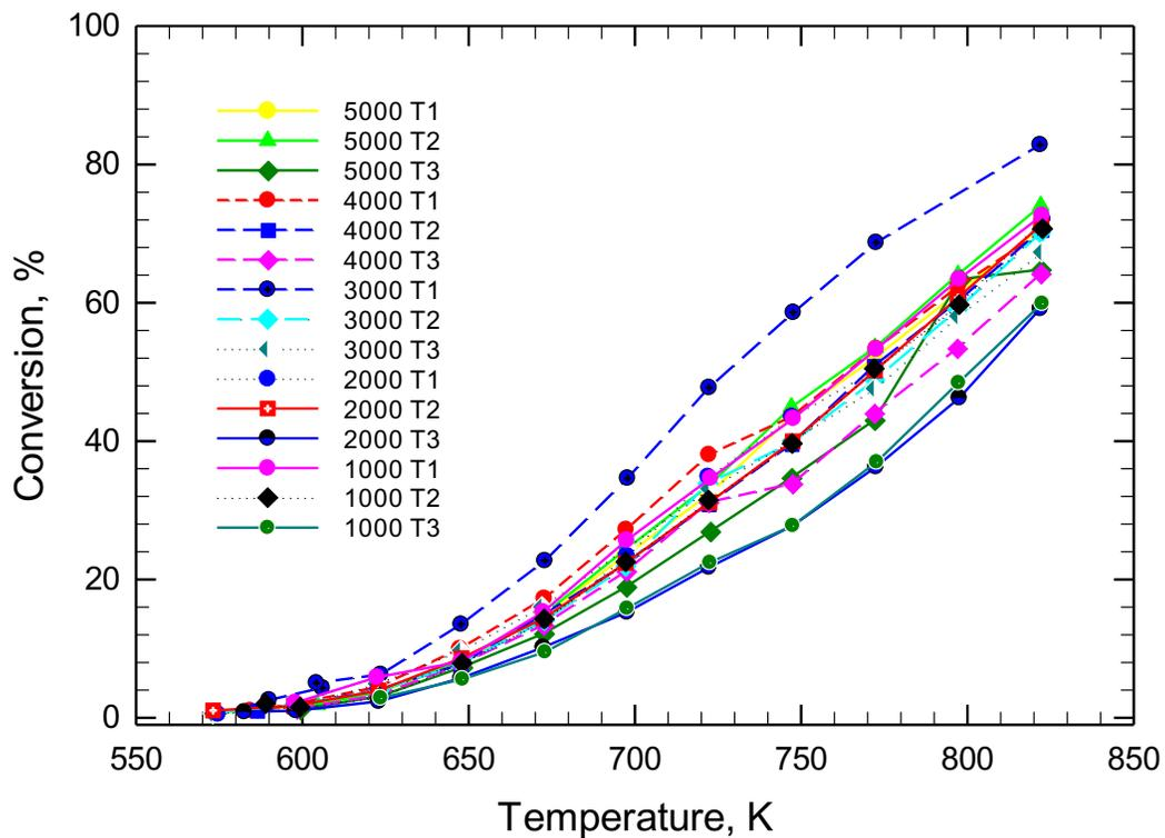
Figure 3.8 Ignition curves for  $\text{Co}_3\text{O}_4$  catalyst for three trials (T1-T3) at different  $\text{CH}_4$  concentrations (ppmv), 10 vol.%  $\text{H}_2\text{O}$ , 0.6 g, 210  $\text{mL}_{\text{STP}}/\text{min}$ , 19.5 vol.%  $\text{O}_2$ ,  $\text{GHSV} = 21,000 \text{ L}_{(\text{STP})}/(\text{kg}_{\text{cat}} \cdot \text{h})$ . The exceptional 3000 T1 run was the first run in the series with 10% water. The order of the trials is shown in Table 1 in the main text.
