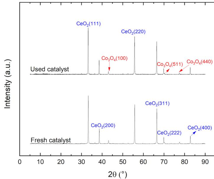
Figure 5.1 XRD profiles of the fresh and used  $\text{Co}_3\text{O}_4/\text{CeO}_2$  (8.6 wt.% Co) catalysts.
