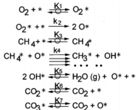
Scheme 1.2. Reaction mechanism of methane combustion on Pd, where \* are unsaturated metal atoms from scheme 1.1. Reprinted from [13] with permission from Elsevier copyright 1998.
