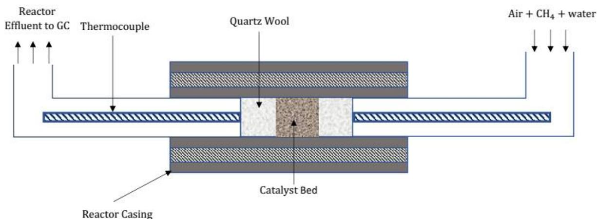
Figure 2.1 Schematic of the reactor system.
