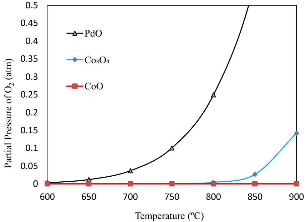
Figure 1.5 Equilibrium oxygen pressure for R3,R4 and R5 phase transformation calculated using expressions presented in [62].
