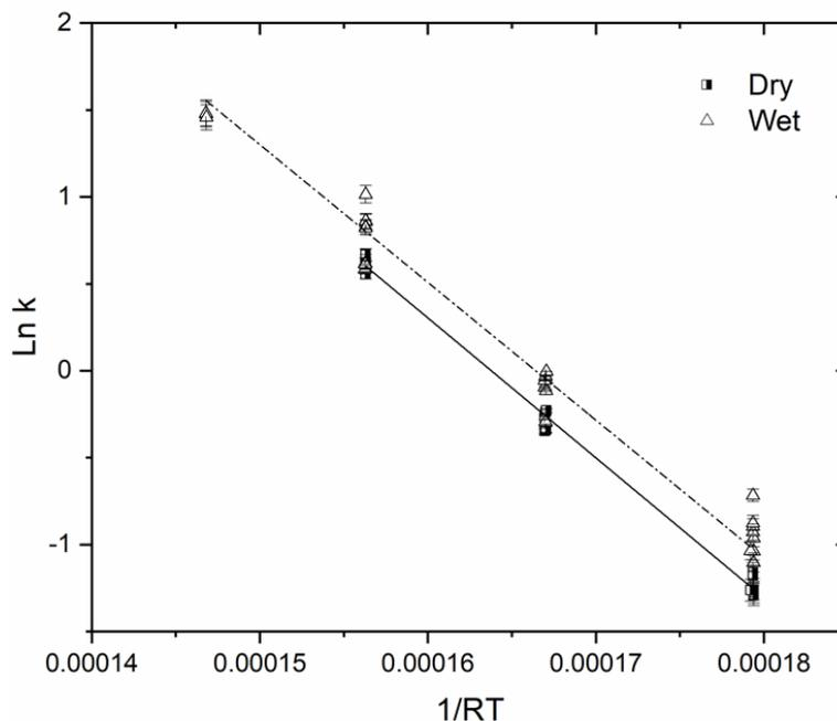
Figure 5.5 Arrhenius plot obtained for combined data at dry and wet conditions.
