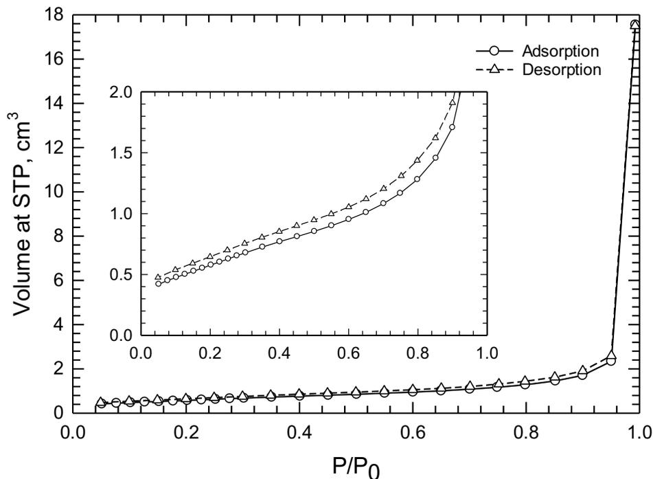
Figure 3.3  $N_2$  adsorption-desorption isotherms measured for the spent  $Pd/Co_3O_4$  catalyst. The inset graph highlights the hysteresis observed at low adsorbed volume.
