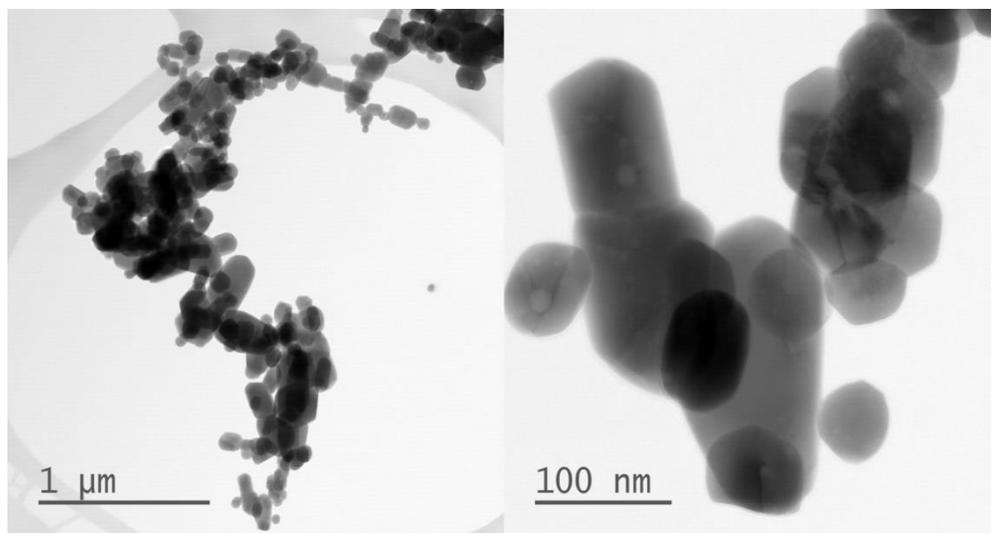
Figure 3.2 TEM images of the spent Co<sub>3</sub>O<sub>4</sub> catalyst.
