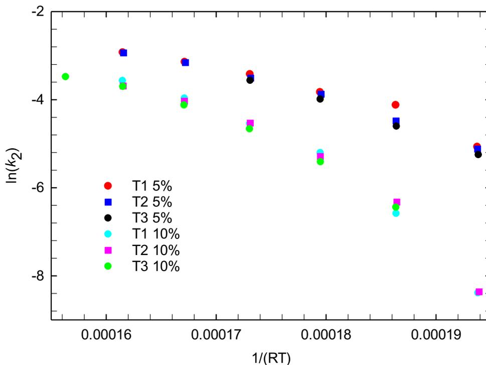
Figure 3.7 . Verification of additive Pd and  $\text{Co}_3\text{O}_4$  contribution hypothesis by computing rate constants for Pd component only. The non-linearity rejects the hypothesis and suggests strong metal-support interactions.
