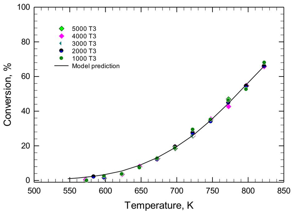
Figure 3.9 Model prediction (first order in  $\text{CH}_4$ ) for the ignition curves on  $\text{Co}_3\text{O}_4$  with 5 % water in the feed for trials (top) T1 and (bottom) T3. See Figure 3.8 caption for the reaction conditions.
