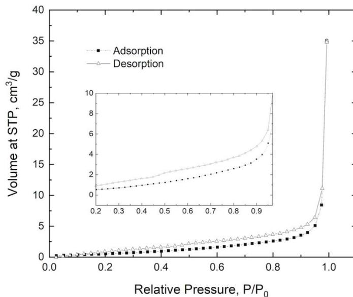
Figure 5.2  $\text{N}_2$  adsorption-desorption isotherms for the fresh (calcined)  $\text{Co}_3\text{O}_4/\text{CeO}_2$  catalyst.
