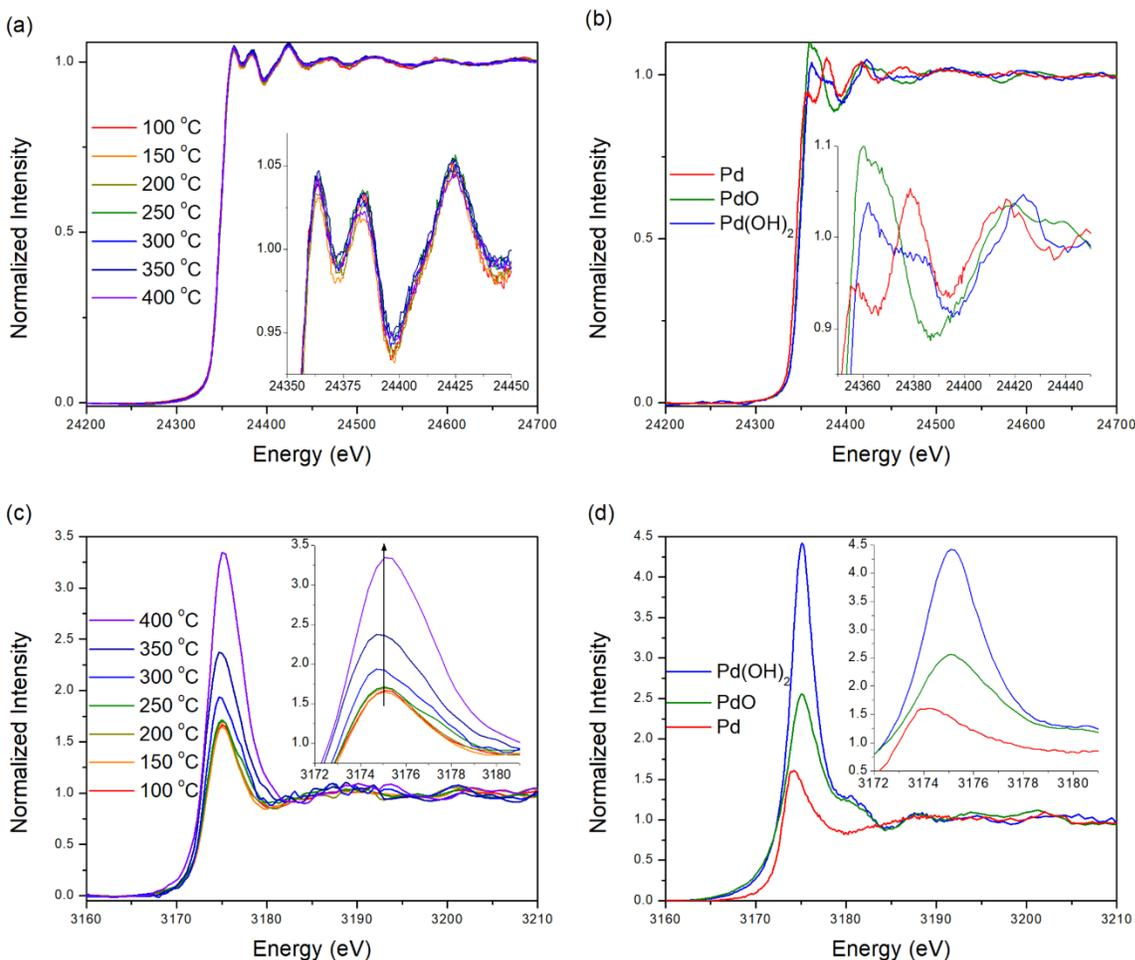
Figure 4.8 (a) Pd K edge XAS spectra of Pd/CoO<sub>x</sub> catalyst under *in situ* wet methane oxidation conditions and (b) Pd K edge standards; (c) Pd L<sub>3</sub> edge of the Pd/Co<sub>3</sub>O<sub>4</sub> catalyst *in situ* and (d) Pd L<sub>3</sub> edge standards.
