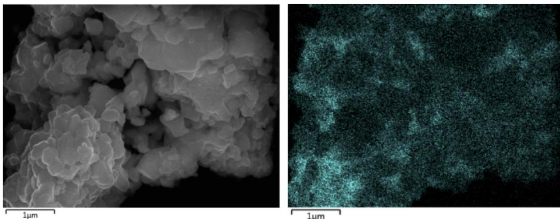
Figure 5.3 Scanning electron micrograph (left) and cobalt distribution (right) for the used  $\text{Co}_3\text{O}_4/\text{CeO}_2$  catalyst.
