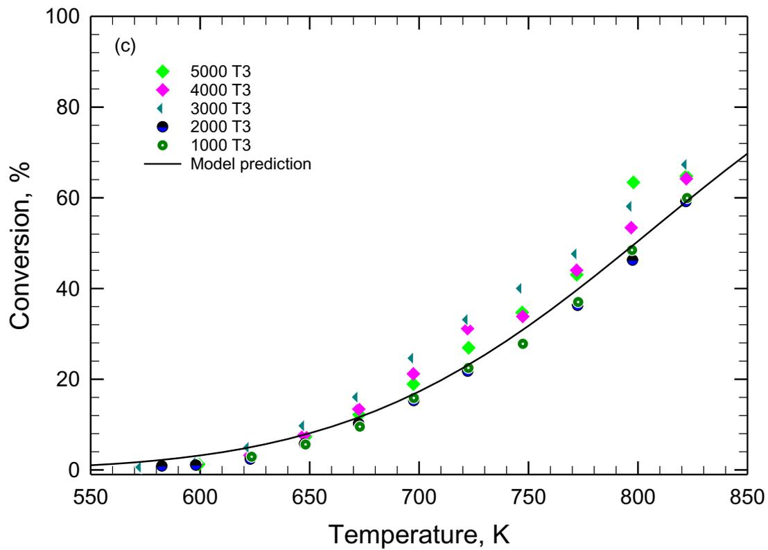
Figure 3.10 Model prediction (first order to  $\text{CH}_4$ ) for the ignition curves on  $\text{Co}_3\text{O}_4$  with 10% water in the feed for trials (a) T1, (b) T2 and (c) T3. See Figure 3.8 for the reaction conditions.
