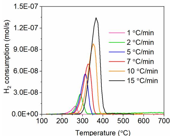
Figure 4.2 TPR profile of  $\text{Co}_3\text{O}_4$  (0.0026 g) in  $\text{H}_2$ . The  $\text{H}_2$  consumption is monitored by a calibrated on-line mass spectrometer.
