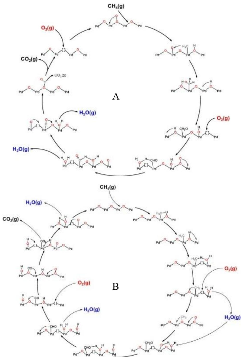
Figure 1.2 Catalytic cycle of the preferential reaction path following a Mars-van-Krevelen redox mechanism for methane oxidation over PdO(1 0 1) as found at (A) dry feed (200–400 °C) and (B) wet feed (12%  $\text{H}_2\text{O}$ , 300–550 °C). Reprinted from [35] with permission from Elsevier copyright 2019.
