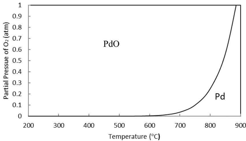
Figure 1.4 Equilibrium O<sub>2</sub> pressure for Pd ⇌ PdO transformation
