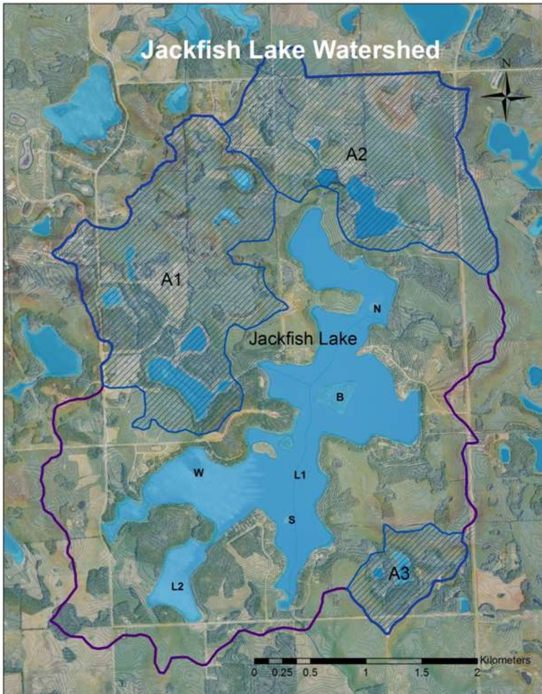
Figure 45. Effective and gross drainage areas for Jackfish. The dark blue line delineates the gross drainage area. Section A1, A2, and A3 are considered non-contributing. L2 and connects to L1 and as such is considered to be part of the effective drainage area. Islands are labelled B, N, S and W (Sal Figliuzzi and Associates, 2016).
