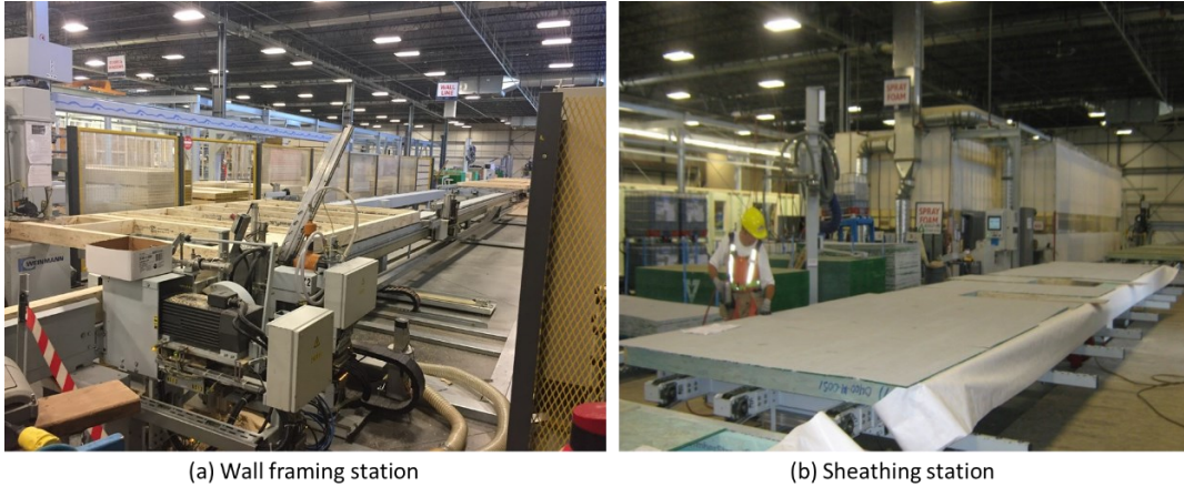
Figure 3.1. (a) Framing (b) Sheathing stations of wall production line (ACQBUILT Inc. 2019).
