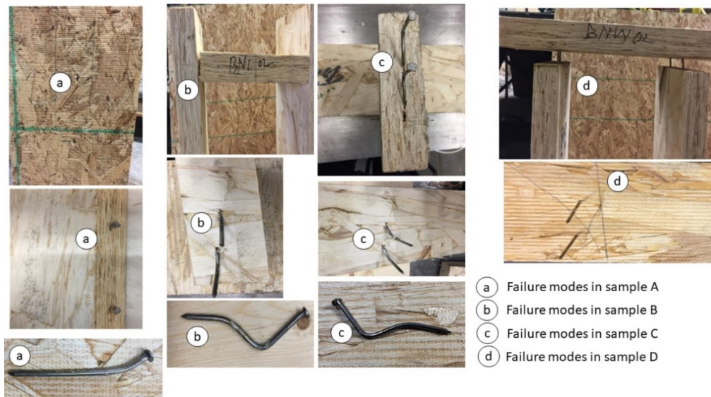
Figure 2.16. Failure modes of nail connections under monotonic loading
