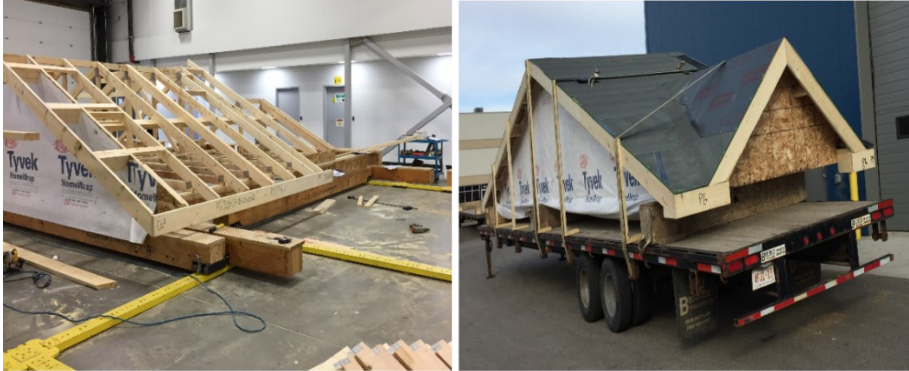
Figure 5.1. Present state of roof production (a) Truss layout (b) Loaded roof component unit.
