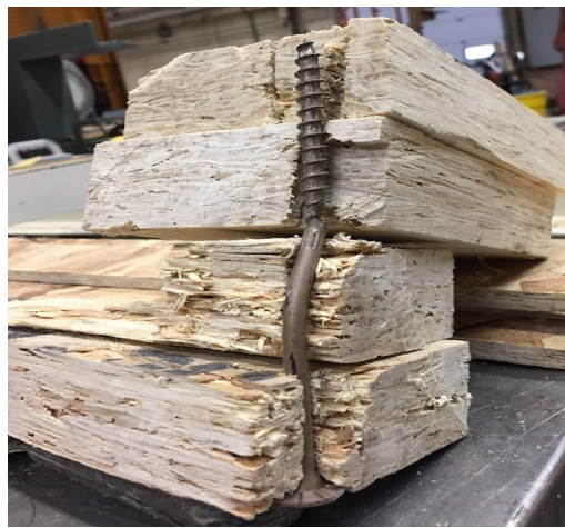
Figure 3.24. Failure mode of Connection-C.
