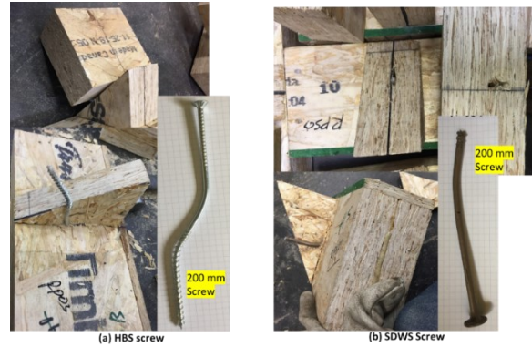
Figure 3.18. Failure of mode of Connection-A in shear loading (a) HBS screw (b) SDWS screw.
