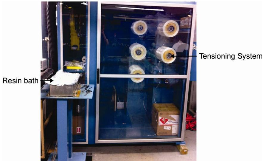
Figure 2.1: Image of the tensioning system and resin bath
