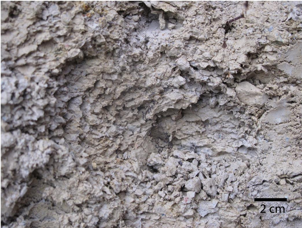
**Fig. 2-3:** Sandy-silt till showing fissility. This photo was taken at 1 m depth from the natural land surface.
