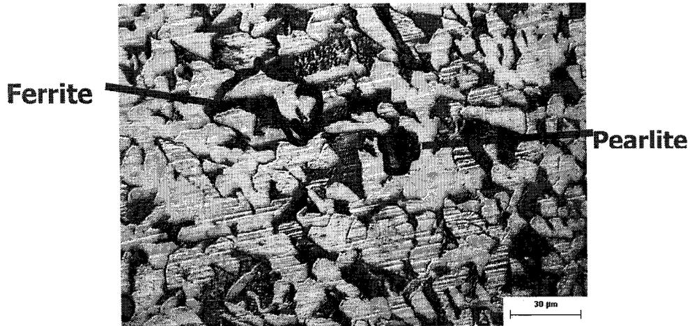
Figure 3-1 Microstructure of X-52 pipeline steel
