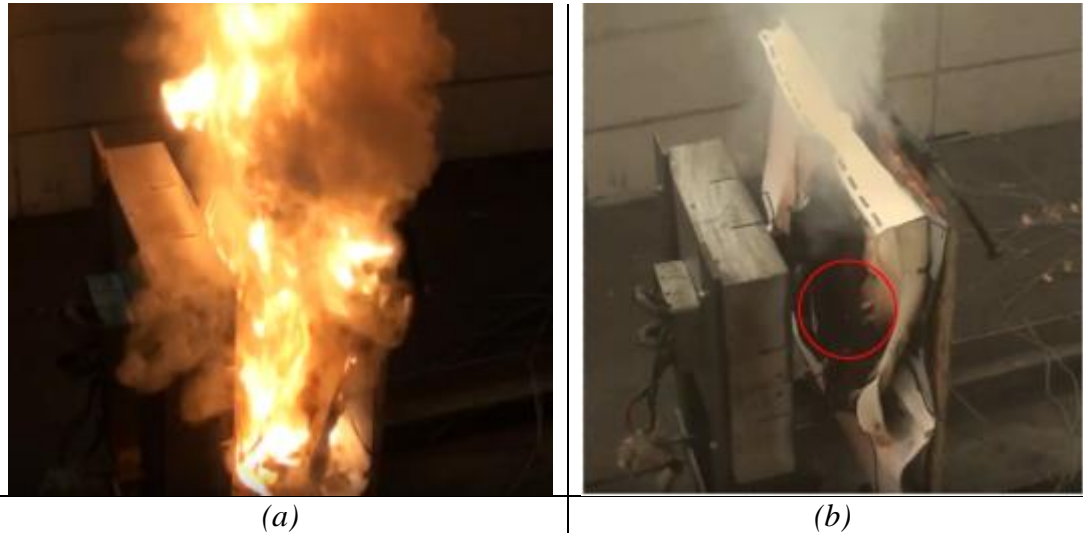
Figure 16 Comparison of the burn tests of the VS prototype under (a) the HHC and (b) the LHC. The red circle indicates the region where glowing ignition was observed.
