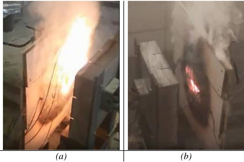
Figure 19 Comparison of the ignition process of the EW prototype under (a) the HHC and (b) the LHC.
