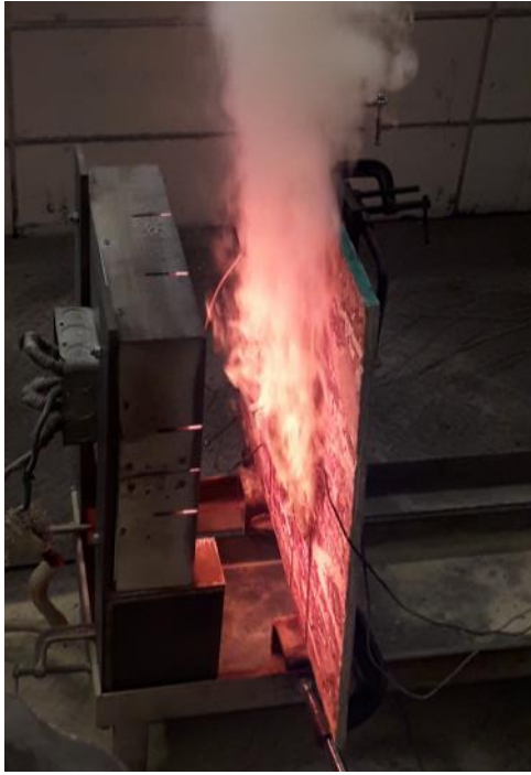
(a) Fuel gases generated at the exposed surface
