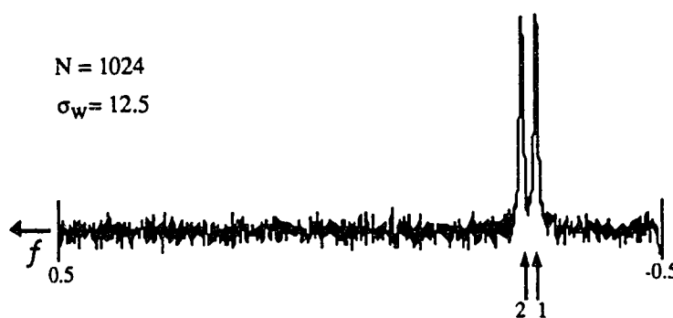
Figure 5.2.1.1 A representative 1024-point DFT spectrum for Examples 5.2.1 to 5.2.3 consisting of two time domain sinusoids of equal amplitude (250), equal damping rate (0.00318) and of normalized frequency separation 0.025. \sigma_w is the noise standard deviation in time domain defined in Equation (1.1.1).
