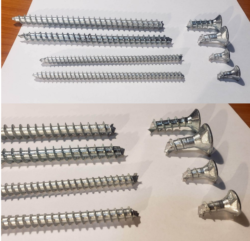
Figure 3-12: Failure in ASSY 8-160, ASSY 10-200, ASSY 12-200 (countersunk head) screws
