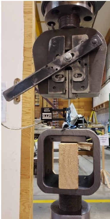
Figure 3-7: Complete screw tensile test setup
