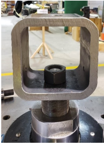
Figure 3-5: The adapter made from a steel channel section with a hole in the middle to accommodate the screw
