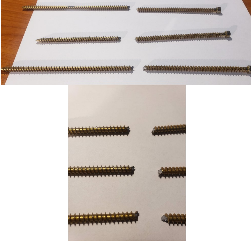
Figure 3-11: Failure in ASSY 6-200 (cylindrical head) screws
