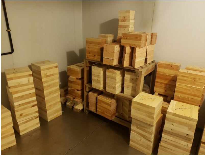
Figure 6-2: Conditioning of samples in a conditioning chamber
