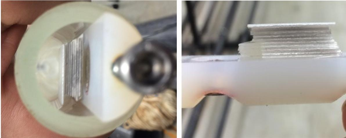
**Figure 3-16 Calibration target base with calibration grid attached to it**
