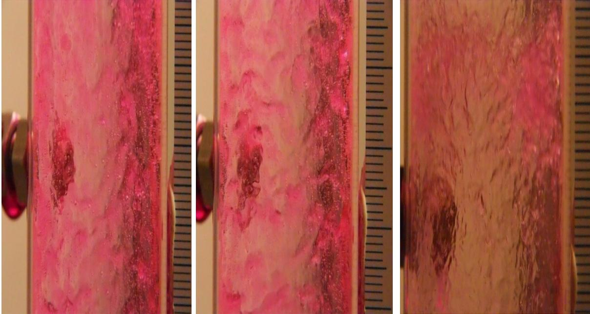
**Figure 4-12 Images taken with high speed camera at 60 LPH of liquid flow rate and at 800, 900 and 1100 SLPM of gas flow rates**
