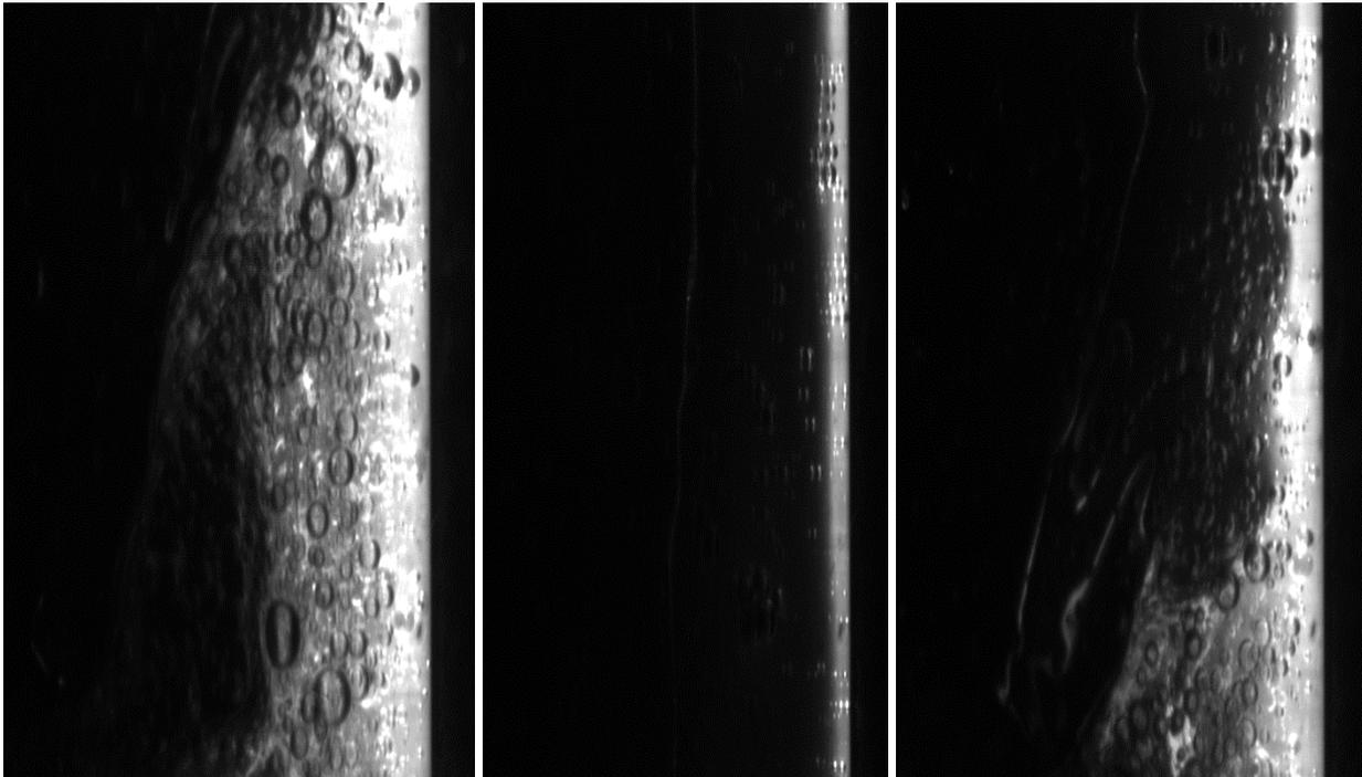
**55 LPH (liquid rate) and 600 SLPM (gas rate) (left to right: maximum, minimum, and average)**
