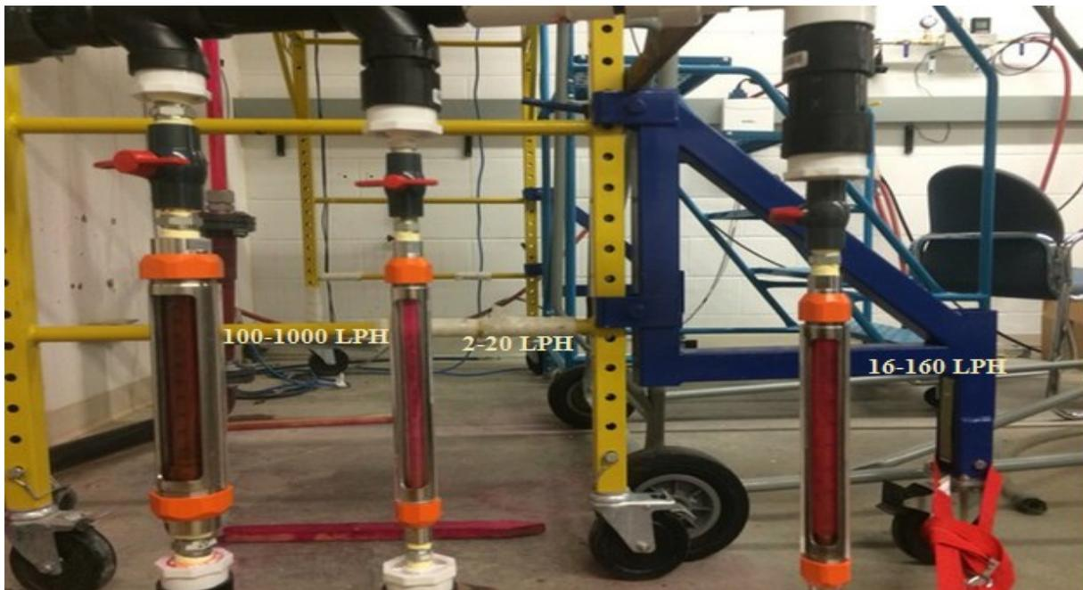
Figure 3-2 Water rotameters with different ranges
