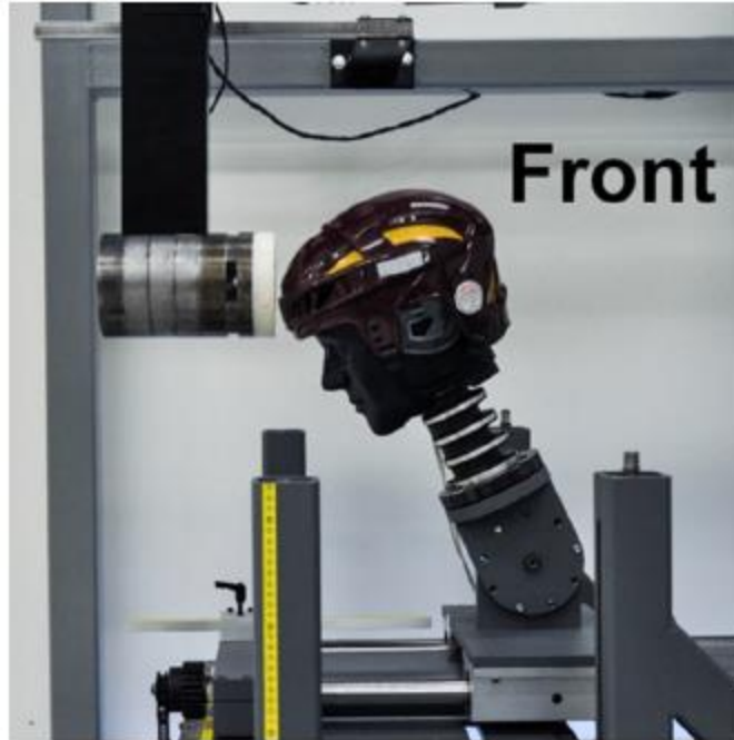
Figure 2.9: Example of Hockey STAR helmet assessment metric setup of forehead pendulum impact tests
