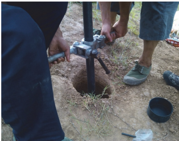
Figure 3.3: Pulling of thin-wall tube
