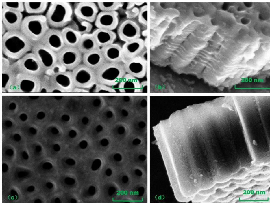
Figure 2- 9 FESEM images of TNTAs anodized at 40 V for 20 min (a) Top view and (b) Cross-section for samples annealed at 500°C for 2.5 hours;(c) Top-view and (d) Cross-section for samples annealed at 750 °C for 2.5 hours.
