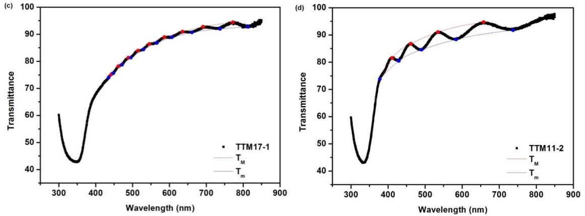
Figure 3- 3 Transmittance spectra measured from (a) blank glass, (b) TNTAs TTM 16-3, (c) TNTAs TTM 17-1, and (d) TNTAs TTM 11-2, and construction of envelopes in the TNTAs transmittance spectra fringes.
