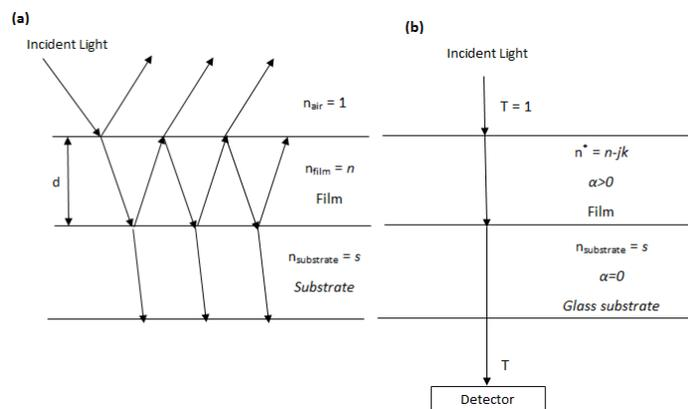
Figure 3- 1 Schematic sketch of the typical behavior of light passing through a thin film
