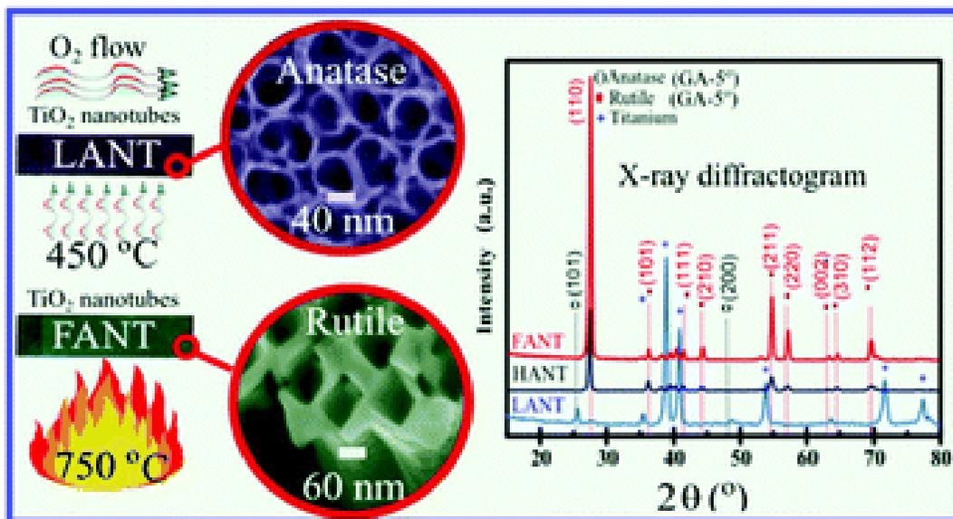
Figure 2- 5 Flame annealing of anatase TiO<sub>2</sub> nanotubes to produce rutile phase TiO<sub>2</sub> nanotubes. FANT mean flame annealed TiO<sub>2</sub> nanotubes and LANT stands for low-temperature annealed TiO<sub>2</sub> nanotubes. Reprinted from [54] with permission from Royal Society of Chemistry.
