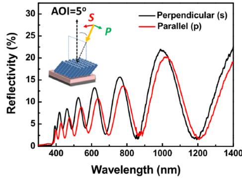
Figure 1- 8 Reflectivity spectra of the oblique-aligned ZnO NWAs for s- and p-polarization at the AOI of  $5^\circ$ . The plane of incidence is aligned to the orientation of NWs. The s- and p-polarization is perpendicular and parallel to the azimuthal direction of the long axis of obliquealigned NWAs, respectively. Reprinted from [30] with permission from Optical Society of America.
