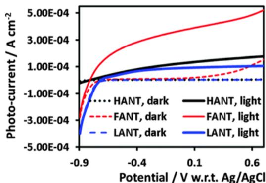
Figure 1- 3Photoelectrochemical water splitting performance by rutile and anatase TNTAs. Reprinted from [26] with permission from Royal Society of Chemistry.
