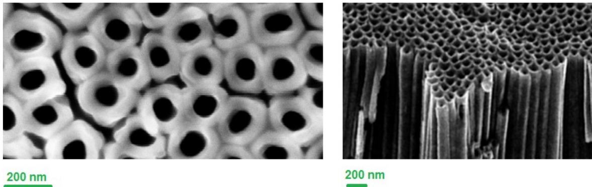
Figure 1- 7Top view (left) and cross section (right) of TNTAs on native substrate.
