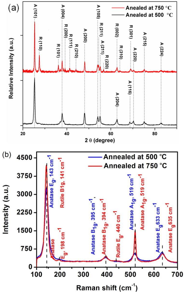
Figure 2- 10 (a) XRD patterns and (b) Raman spectra of TNTAs anodized at 40 V for 20 min and furnace annealed at 500 °C and 750 °C for 2.5 hours.
