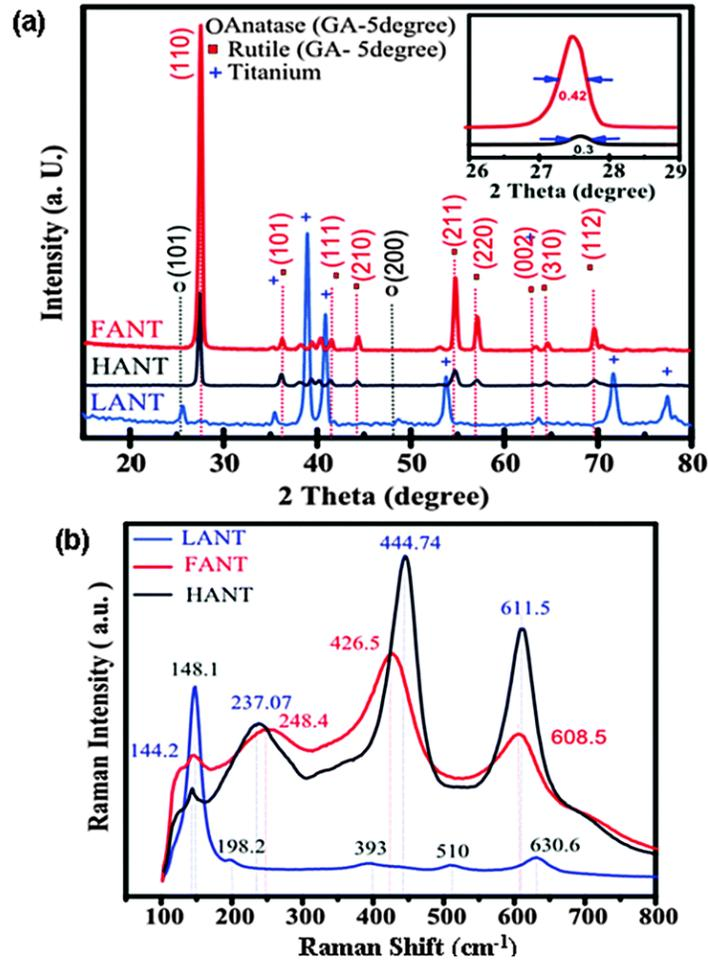
Figure 2- 7 XRD and Raman spectra of LANTs, HANTs and FANTs. Reprinted from [54] with permission from Royal Society of Chemistry.
