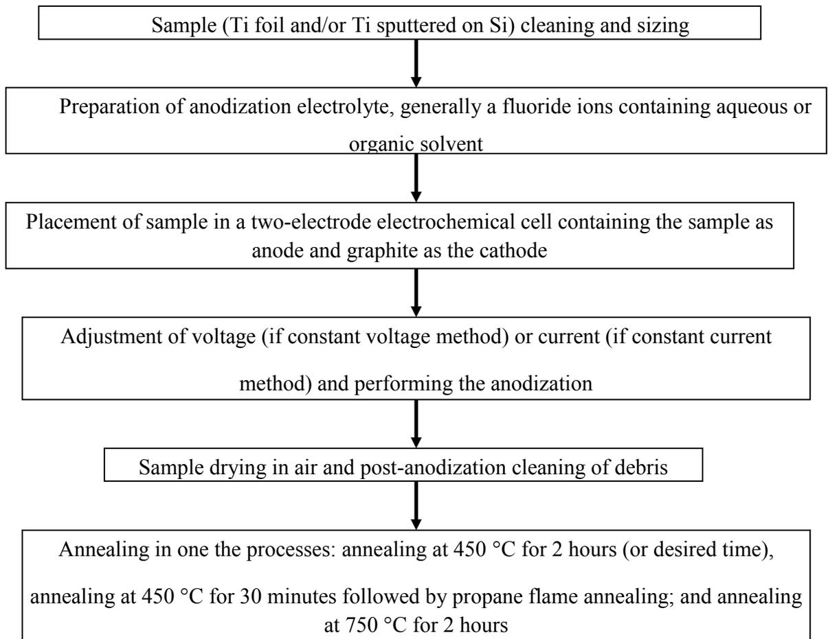
Figure 2- 3Process flow for fabrication of anodic TiO<sub>2</sub> nanotubes followed by appropriate annealing procedure.
