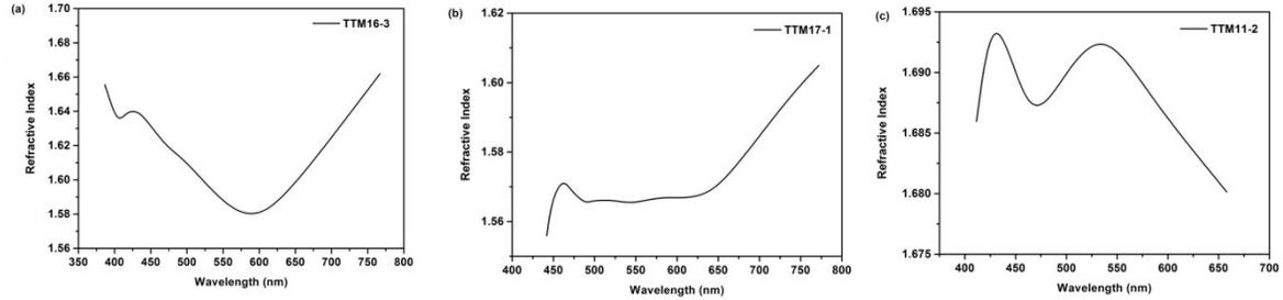
Figure 3- 4Refractive indicesof (a) TNTAs TTM 16-3, (b) TNTAs TTM 17-1, and (c) TNTAs TTM 11-2 obtained using Swanepoel’s method.
