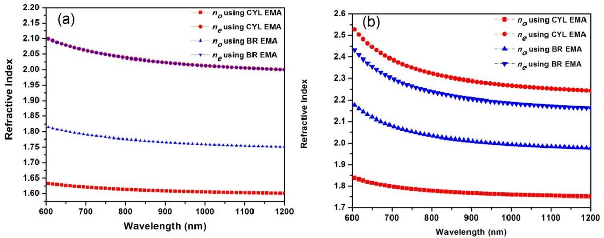
Figure 4- 3 Anisotropic refractive index of TNTAs constituted by (a) Anatase-phase  $\text{TiO}_2$  and (b) Rutile-phase  $\text{TiO}_2$ , calculated using the BR and CYL effective medium approximations, see Eqns (1) through (6).
