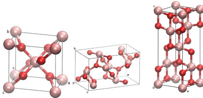
Figure 1- 1 Titanium dioxide crystal structures of rutile, brookite and anatase (from left to right). Reprinted from [4] with permission from IOP Publishing Ltd.
