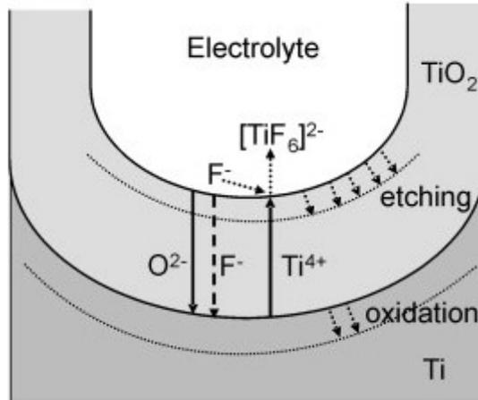
Figure 2- 1 Illustration of the anodic TNTAs growth in presence of fluorides. Reprinted from[41] with permission from Elsevier.
