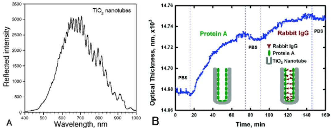
Figure 1- 4TNTA-based interferometric biosensors: (A) representative reflectivity spectrum of anodic TNTAs showing the characteristic interference fringes and (B) Time-dependent optical thickness measurements showing sequential binding of Protein A and rabbit IgG within TNTAs. Reprinted from [27] with permission from Springer Netherlands.
