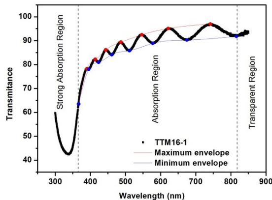
Figure 3- 2 Transmission spectrum a TNTAs sample anodized in 4 vol% water and 0.3
