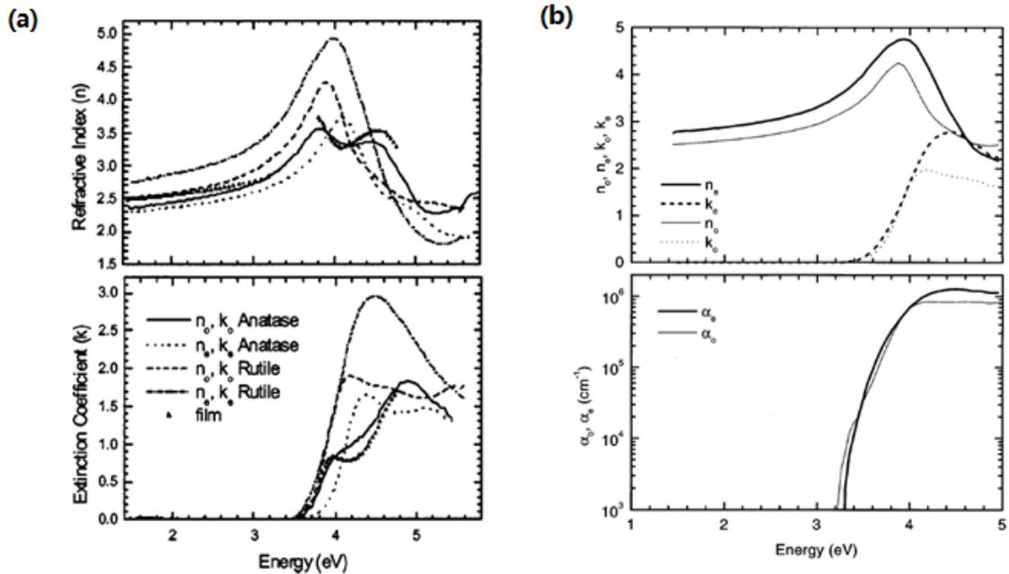
Figure 1- 6 (a) the refractive index and extinction coefficient bulk anatase, rutile, and thin-film anatase determined from the spectroscopic ellipsometry data. (b)optical functions of bulk. Top, real and imaginary parts of the complex refractive index for the ordinary and the extraordinary directions; bottom, absorption coefficients for the ordinary
