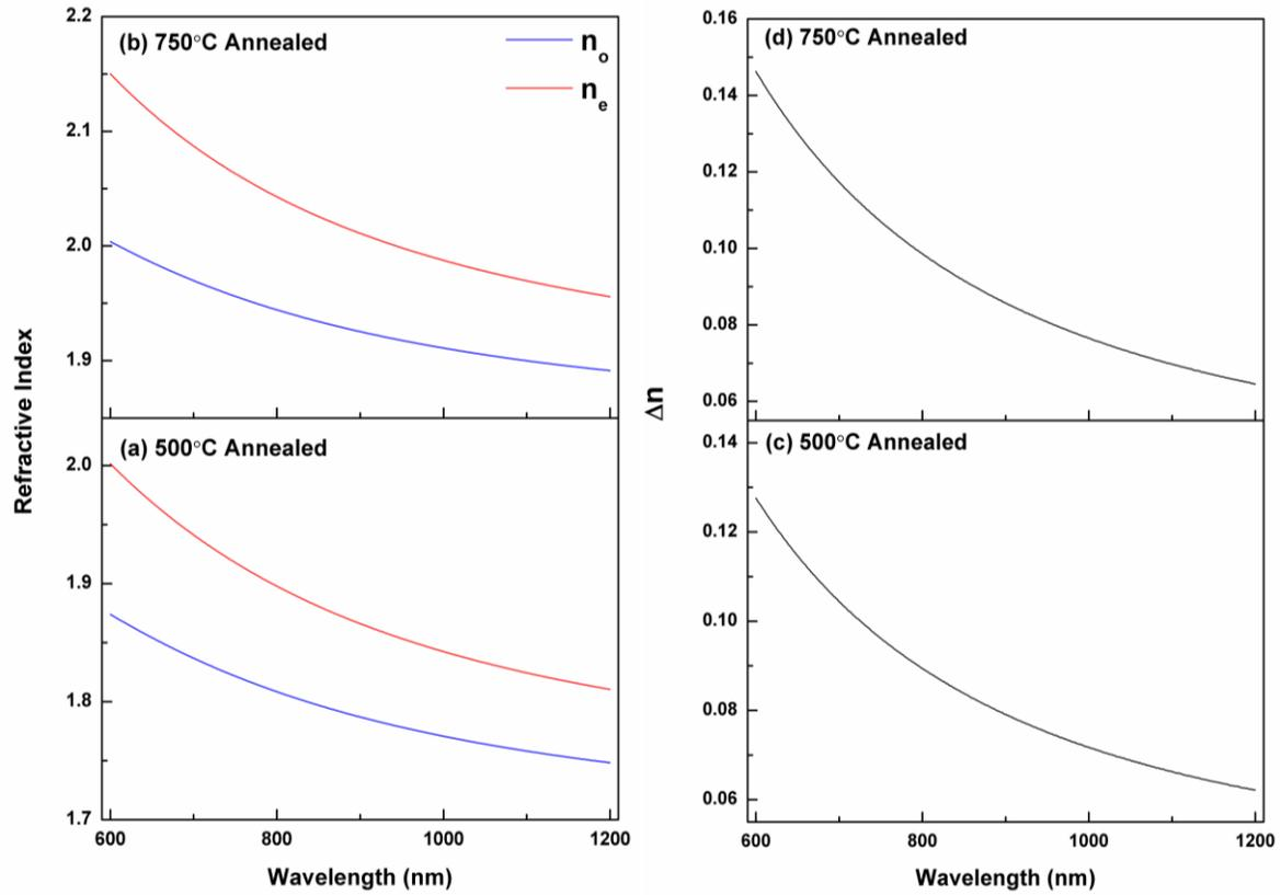
Figure 4- 5 Ordinary and extraordinary refractive indices dispersion pattern of (a) anatase TNTAs and(b) rutile+anatase mixed-phase TNTAs. And birefringence dispersion patterns for (c) anatase TNTAs and(d) rutile+anatase mixed-phase TNTAs.
