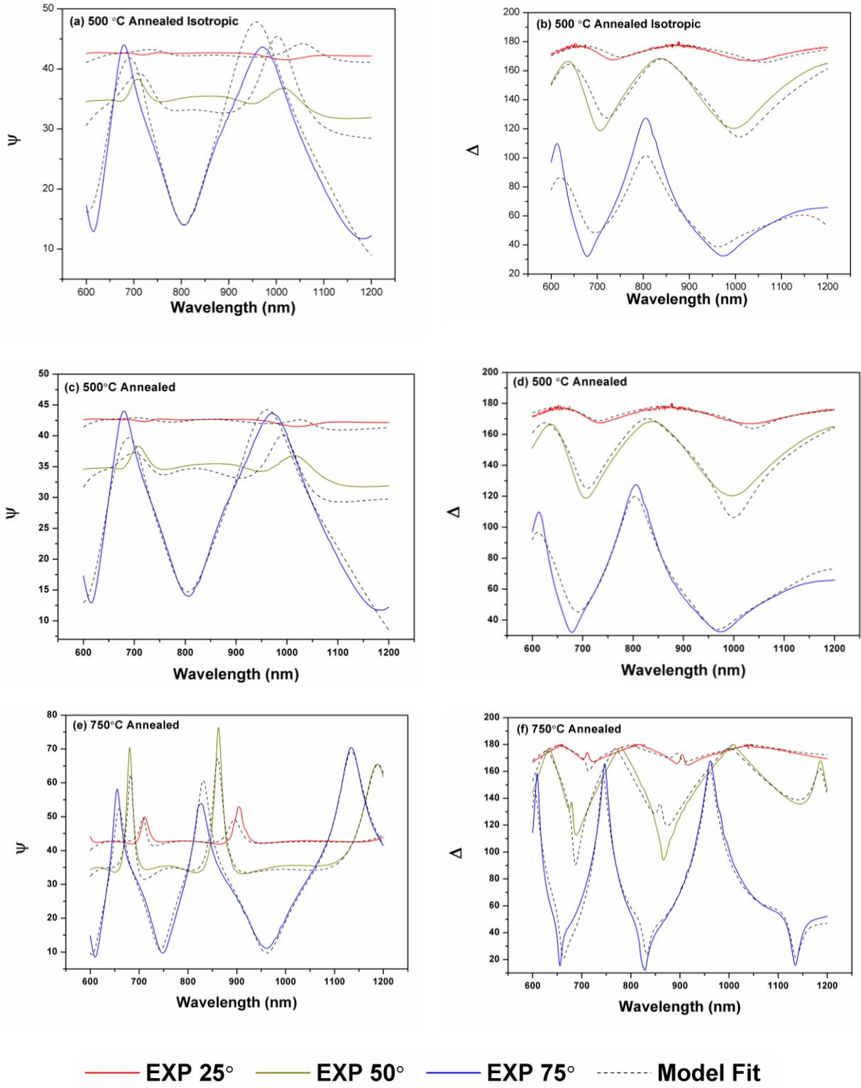
Figure 4- 4Ellipsometric dispersion patterns including measured experimental data (solid lines) and generated curves from best-fit models (dotted lines) for three different angles of
