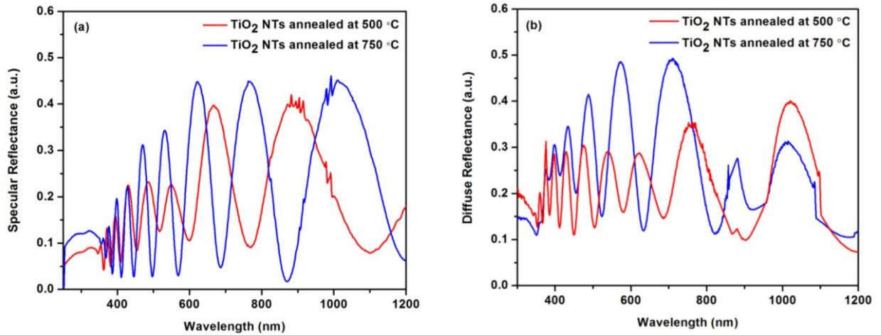
Figure 4- 1(a) Specular and reflection spectra of TNTAs measured in response to unpolarized light incident on the TNTAs at a 20° angle of incidence. The high reflectance values and clear interferometric fringes demonstrate the high optical quality of the TNTA samples. Specular and (b) diffuse reflection spectra of TNTAs measured in response to unpolarized at normal incidence.
