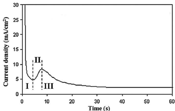
Figure 2- 2 The current-time relation plot for titanium anodized at 20 V. Reprinted from[47]with permission from Wiley-VCH.
