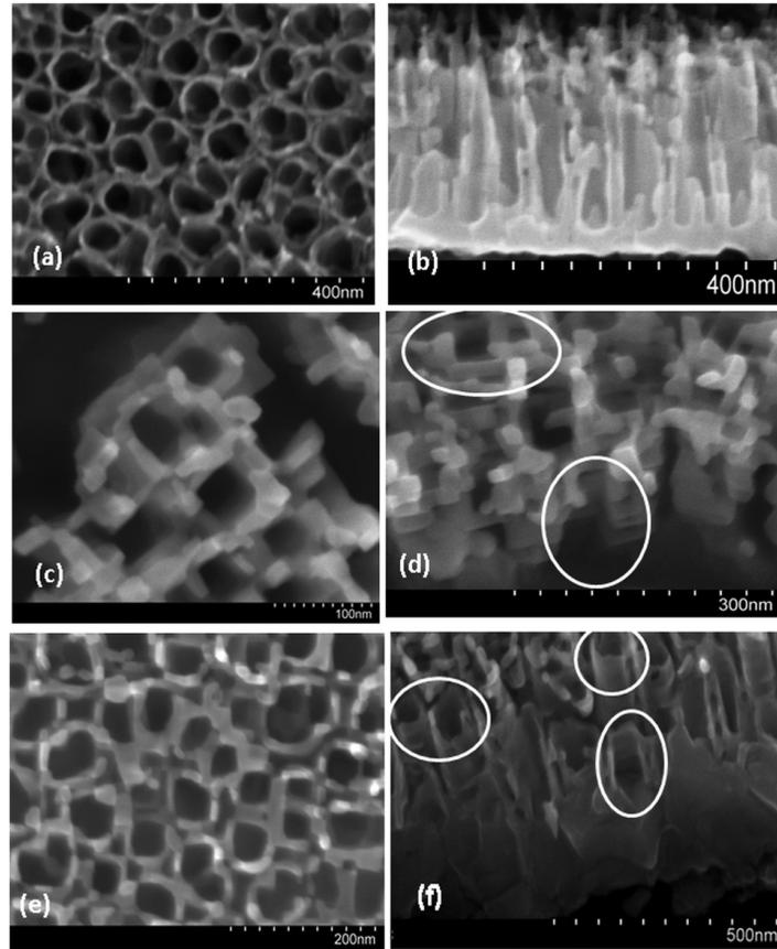
Figure 2- 6 FESEM image of LANTs (a and b), HANTs (c and d) and FANTs (e and f). The circular marks indicate square section from cross-section. Reprinted from [54] with permission from Royal Society of Chemistry.
