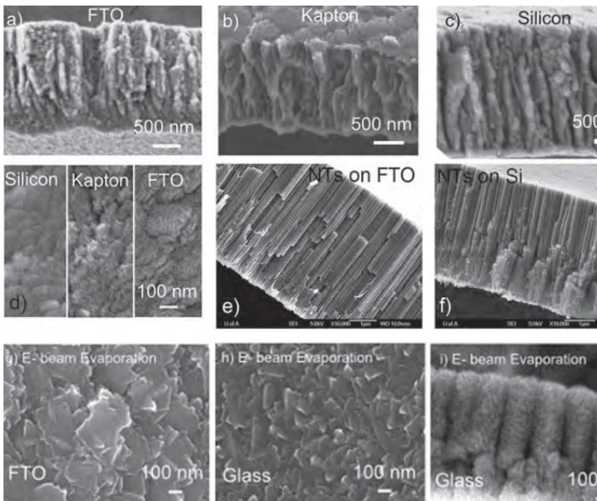
Figure 3- 5 (a–d), (g-i) Cross-sectional and topview of Ti thin films deposited on to glass, FTO coated glass, Kapton and Si wafer substrates respectively; (e, f) ordered TNTAs grown on substrates shown in (a), (c) and (d). Reprinted from [68] with permission from American Scientific Publishers.
