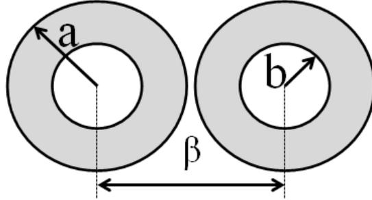
Figure 4- 2 Geometry of the nanotube architecture used in effective medium calculations.
