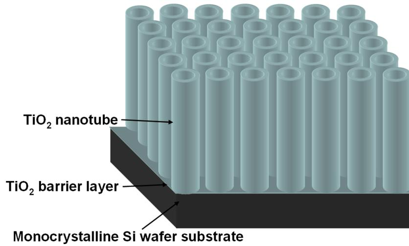
Figure 2- 8 Schematic illustration of anodically formed TiO<sub>2</sub> nanotube arrays on a Si wafer substrate.
