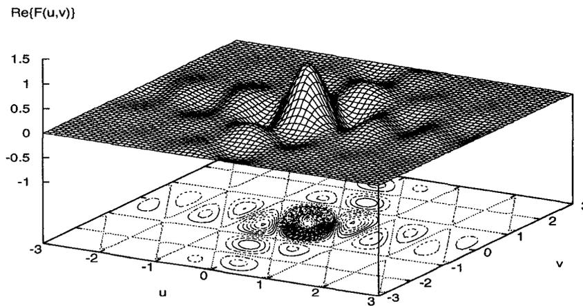
Figure 5.2: The symmetric real-part of the 2-D Fourier transform of the 2-D boxcar function in Figure 5.1.
