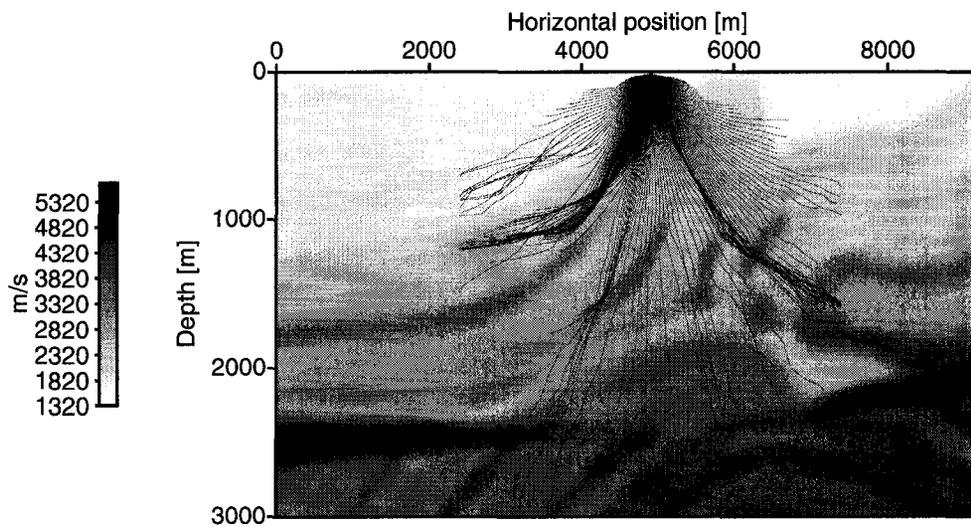
Figure A.1: A sample shot with a ray fan consisting of 161 rays superimposed on the smoothed Marmousi velocity model. Note the shadow zones and caustics. For sufficient coverage with travel-time information extrapolation becomes necessary.
