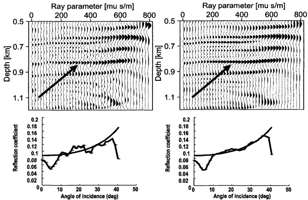
Figure 3.40: Left: Blow-up of the migrated target reflector CIG and the picked AVA curve. Right: Blow-up of the least-squares migrated target reflector CIG (6 iterations) and the corresponding AVA. One has to take care not to produce solutions that are 'too flat'.
