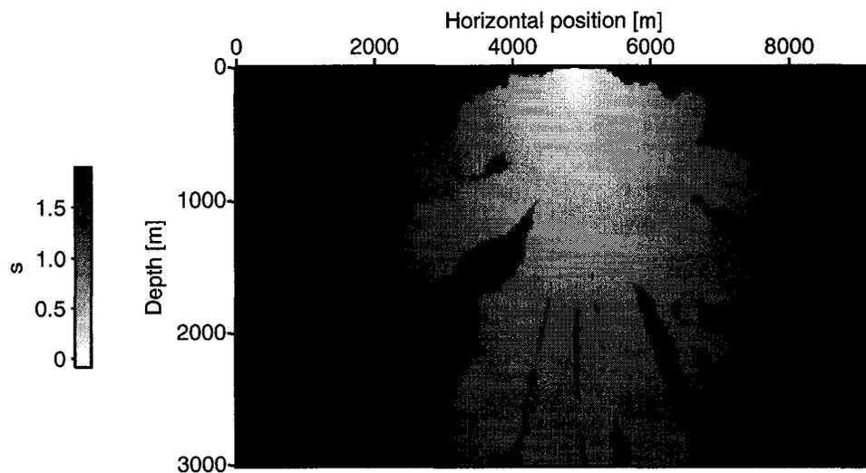
Figure A.2: A sample shot with with rays and travel-times. The travel-times are extrapolated from 161 central rays by a parabolic wavefront approximation (Beydon and Kehe, 1987). The travel-times are given in seconds. The solid areas indicate that no travel-times are available.
