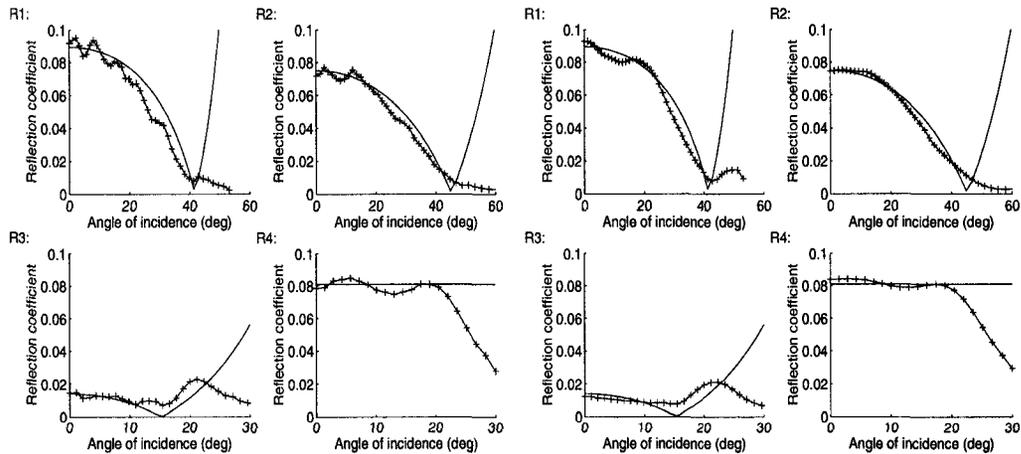
Figure 3.34: Left (R1-R4): AVA picked on the migrated CIG in Figure 3.33 (left). White noise with a signal-to-noise ratio of 10 has been added. Right (R1-R4): The same picks from the least-squares migrated CIG (4 iterations) in Figure 3.33 (right).
