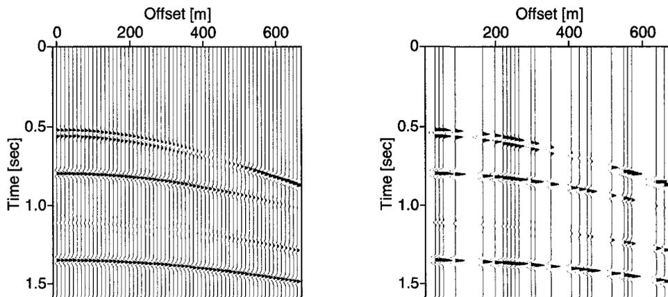
Figure 3.22: Left: CMP gather generated by a ray-tracing code. The code models (cylindrical) geometrical spreading but no transmission effects. The offsets range from 0 to 660 m. The third reflector is about one order of magnitude weaker than the first reflector. Right: The same CMP after randomly removing 50% of the data.
