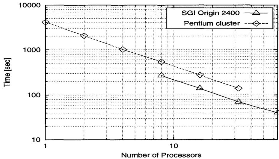
Figure 5.7: Execution times for the parallel computation of the split-step DSR migration of the Marmousi dataset (Figure 3.4). The code has been implemented in a shared-memory (SGI Origin 2400) and a distributed-memory computer architecture (Pentium cluster). Access restrictions to the SGI computer required a minimum usage of 8 processors.
