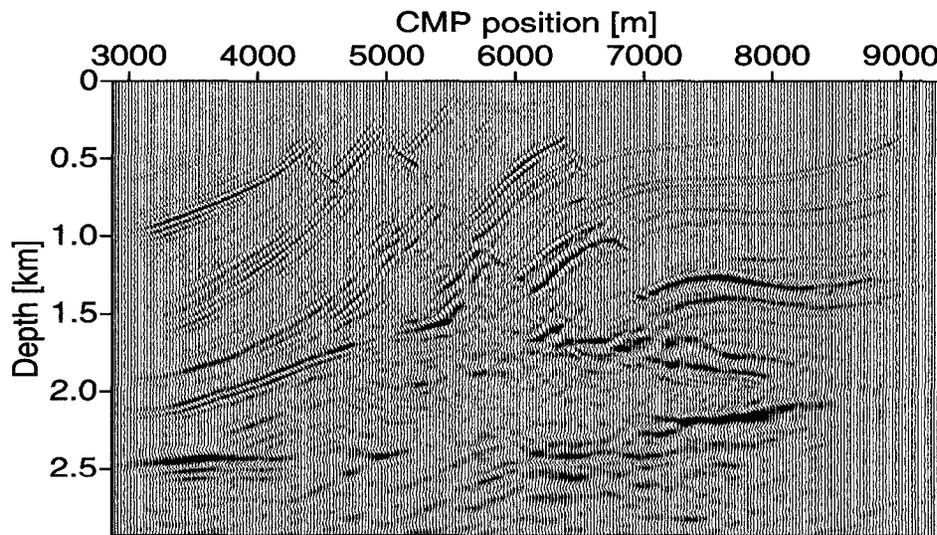
Figure 3.45: Constant ray parameter migration of the Marmousi model ( $p_h = 400\mu\text{s/m}$ ). All available wavefield data were used in the migration.
