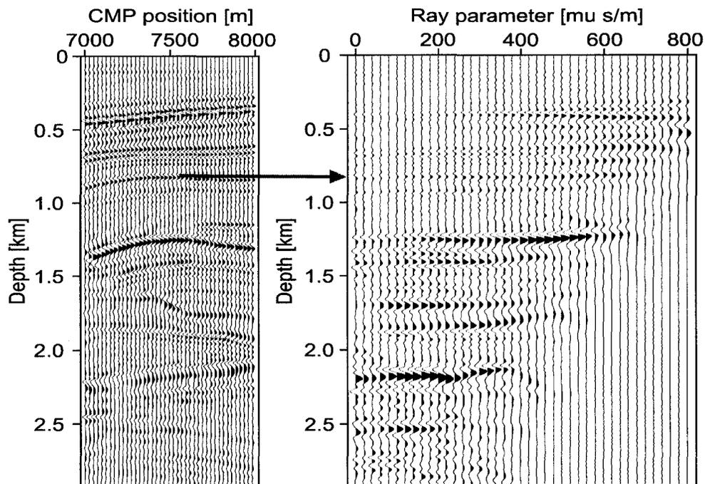
Figure 3.38: Left: Portion of the migrated and stacked Marmousi image. Right: CIG at CMP location 7500 m. The arrow indicates the reflector picked for AVA analysis.
