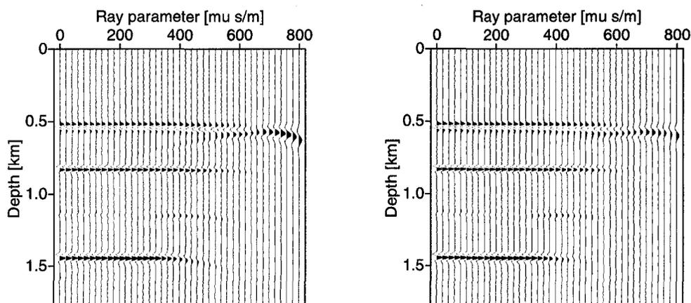
Figure 3.23: Left: Migrated CIG of the complete data. The offset ray parameter axis ranges from 0 to  $800\mu\text{s}/\text{m}$  in steps of  $20\mu\text{s}/\text{m}$ . Right: Least-squares migrated CIG (4 iterations) of the complete data.
