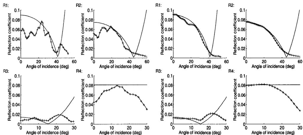
Figure 3.32: Left (R1-R4): AVA picked on the migrated CIG in Figure 3.31 (left). The data were incomplete and random noise with a signal to noise ratio of 10 (based on the absolute maximum amplitude) has been added. Right (R1-R4): The same picks from the least-squares migrated CIG (14 iterations) in Figure 3.31 (right).
