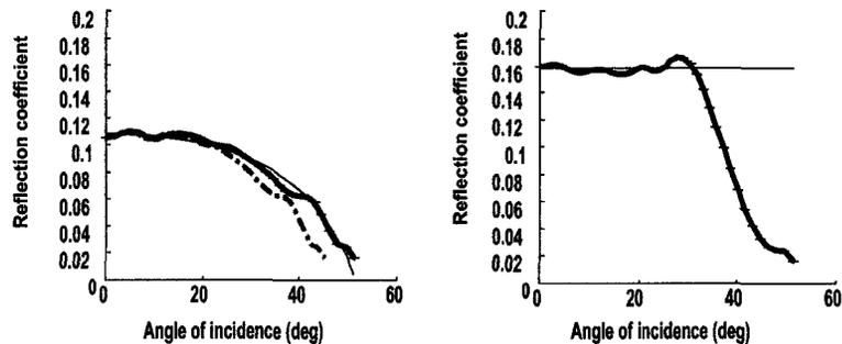
Figure 3.37: Left: AVA for the second reflector picked on the least squares CIG in Figure 3.36. The dot-dashed line indicates the AVA without dip correction. Right: AVA for the third reflector picked on the least-squares CIG in Figure 3.36.
