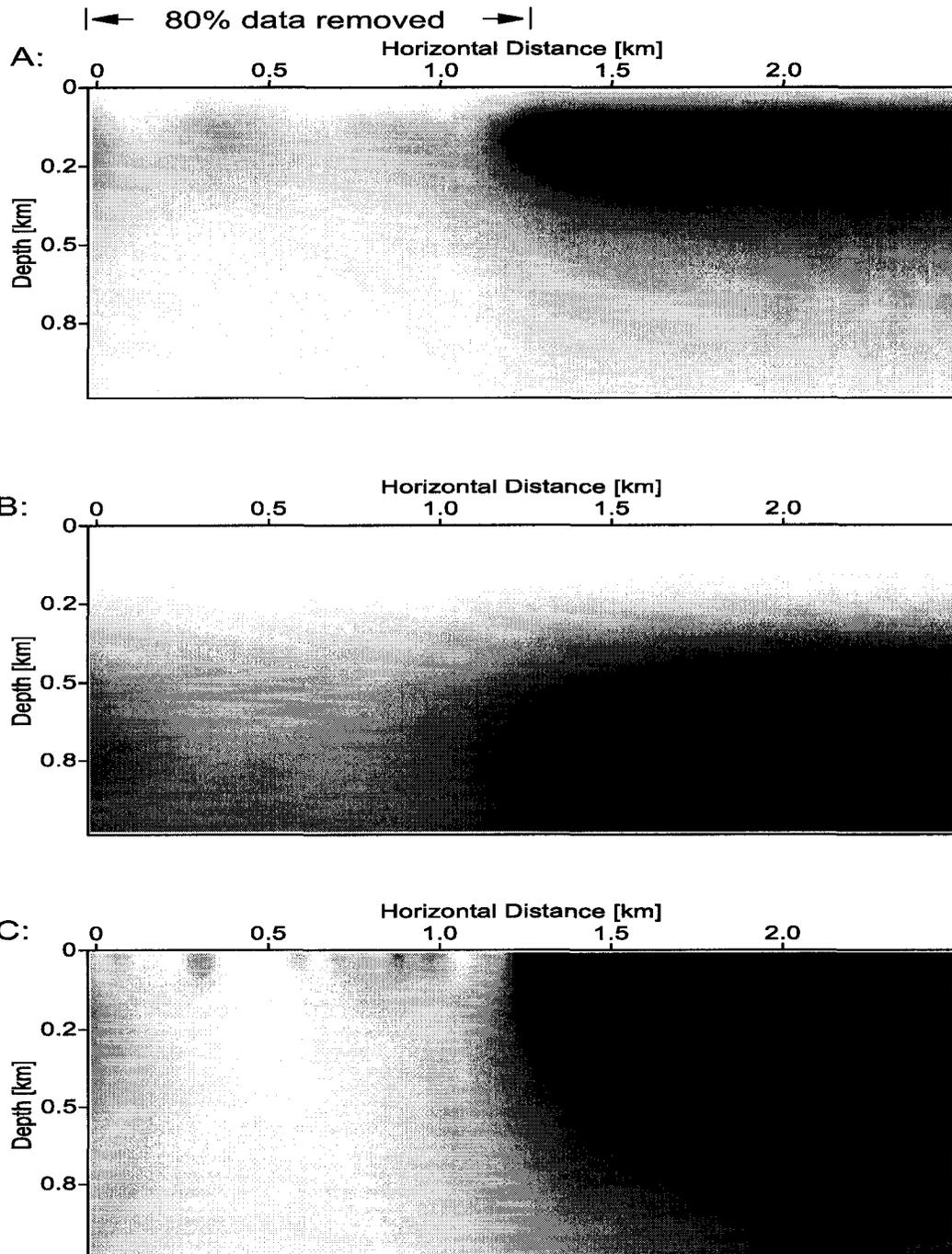
Figure 3.21: Top: Near offset illumination map (100 m). Darker shades mean better illumination. The underlying velocity field increases linearly with depth. Middle: Far offset illumination map (600 m). Far offsets penetrate deeper than the near offsets. Bottom: The illumination map computed for all offsets (0-600 m). The illumination is dominated by the acquisition footprint, especially the near surface.
