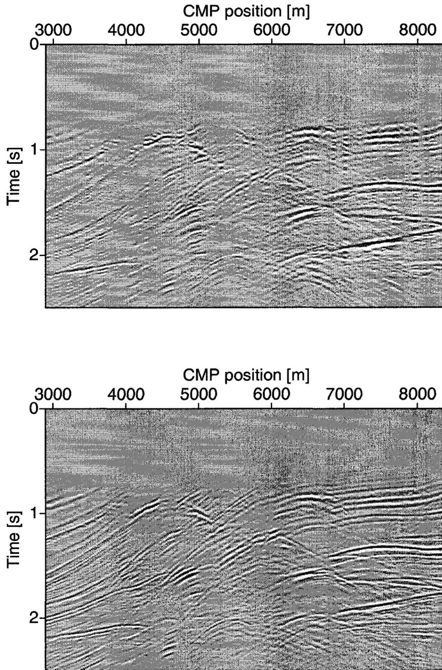
Figure 3.49: Top: Reconstructed constant offset data after one CG iteration based on the incomplete input data in Figure 3.48. Bottom: Reconstructed constant offset data after 12 CG iterations. Notice the wavefront healing effect.
