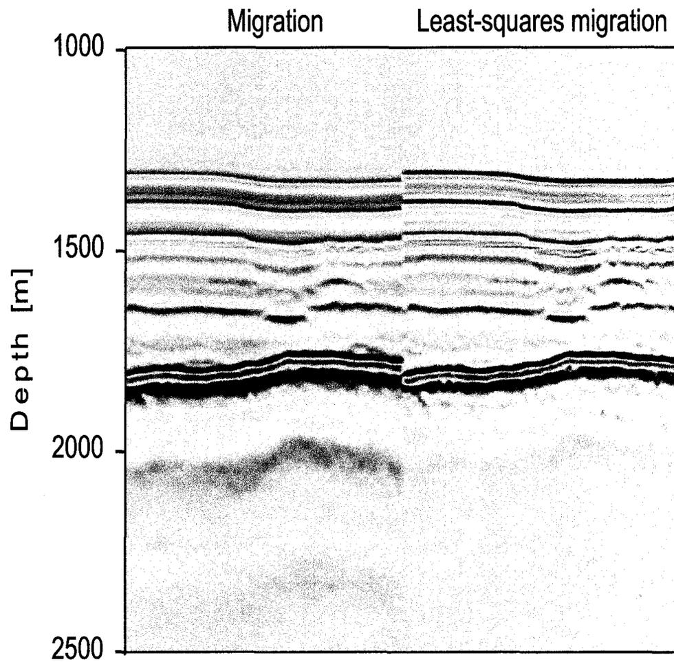
Figure 4.6: Left panel: Parts of the migrated sediment structure and the salt body ranging from 16 km to 17 km in CMP location. Right panel: Least-squares migration of the same area. The amplitudes of both sections are normalized with respect to the prominent top-salt reflector.
