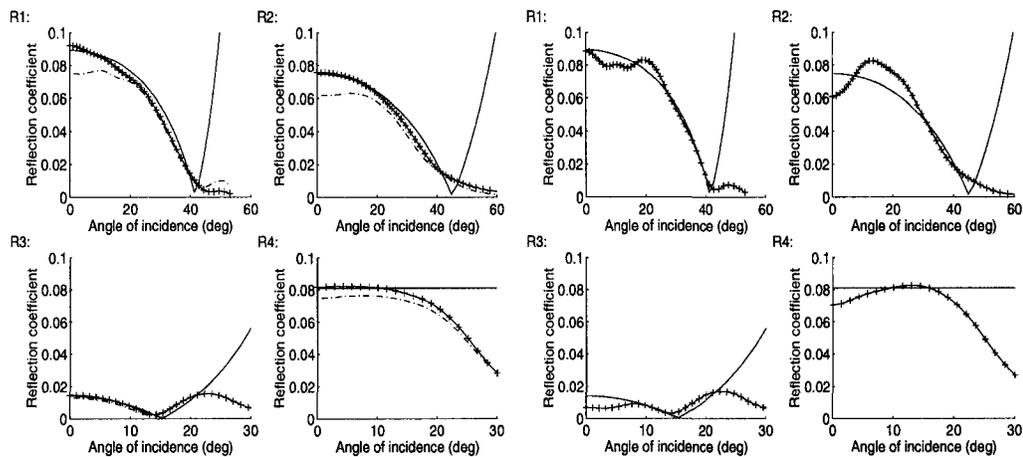
Figure 3.30: Left (R1-R4): AVA picked from the least squares-migrated CIG (10 iterations) in Figure 3.29 (left) shown as the dot-dashed line. The crossed line is the previously shown result after 14 CG iterations. Right (R1-R4): The picks based on the least squares migrated CIG (14 iterations) in Figure 3.29 (right) where the data weighting operator  $\mathbf{W}$  has been replaced by the identity operator.
