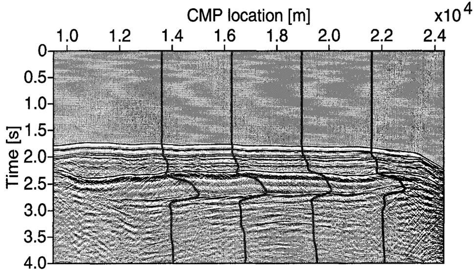
Figure 4.2: Stack after multiple suppression. The first order ocean-bottom multiple has been largely removed. The overlaid curves indicate the CMP positions where velocity profiles have been inverted. The salt body shows as a strong high velocity anomaly in the profiles.
