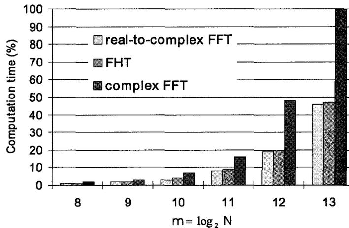
Figure 5.6: Relative computation times for the complex FFT, real-to-complex FFT and FHT as a function of the transform length  $N = 2^m$ . The times have been obtained on a Pentium processor.
