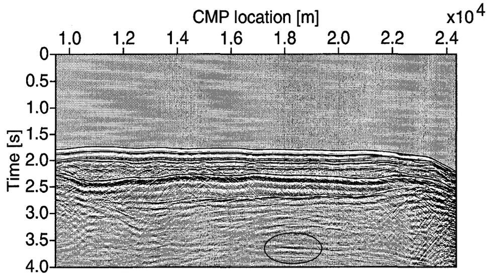
Figure 4.1: Brute-stack of the Gulf of Mexico data. The first-order ocean bottom multiple that partially masks the circled target reflector is easily identified.
