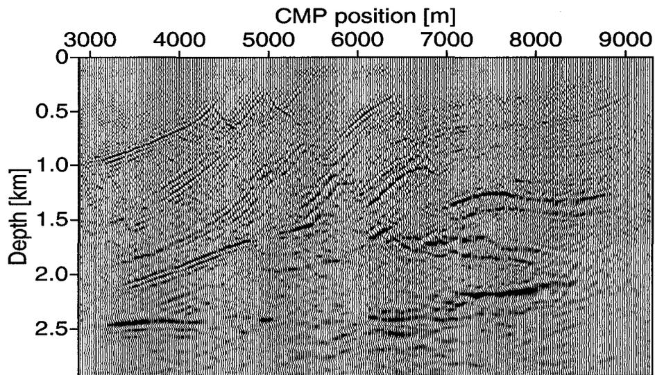
Figure 3.46: Constant ray parameter migration of the Marmousi model ( $p_h = 400\mu\text{s}/\text{m}$ ). Only 30% of the available wavefield data were used in the migration.
