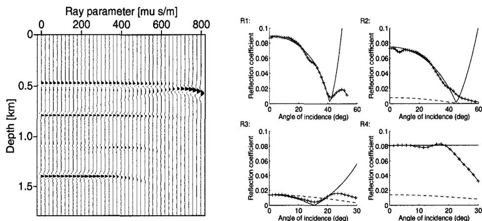
Figure 3.25: Left: Migrated CIG of the complete finite-difference data. As opposed to the ray-tracing data the wavelet has been shifted to be zero-phase. This explains the slightly earlier onset of all signals. Right: The corresponding picked AVA. The dashed line indicates the theoretical cumulative error due to neglected transmission losses.
