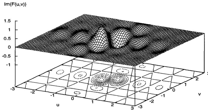
Figure 5.3: The anti-symmetric imaginary-part of the 2-D Fourier transform of the 2-D boxcar function in Figure 5.1.
