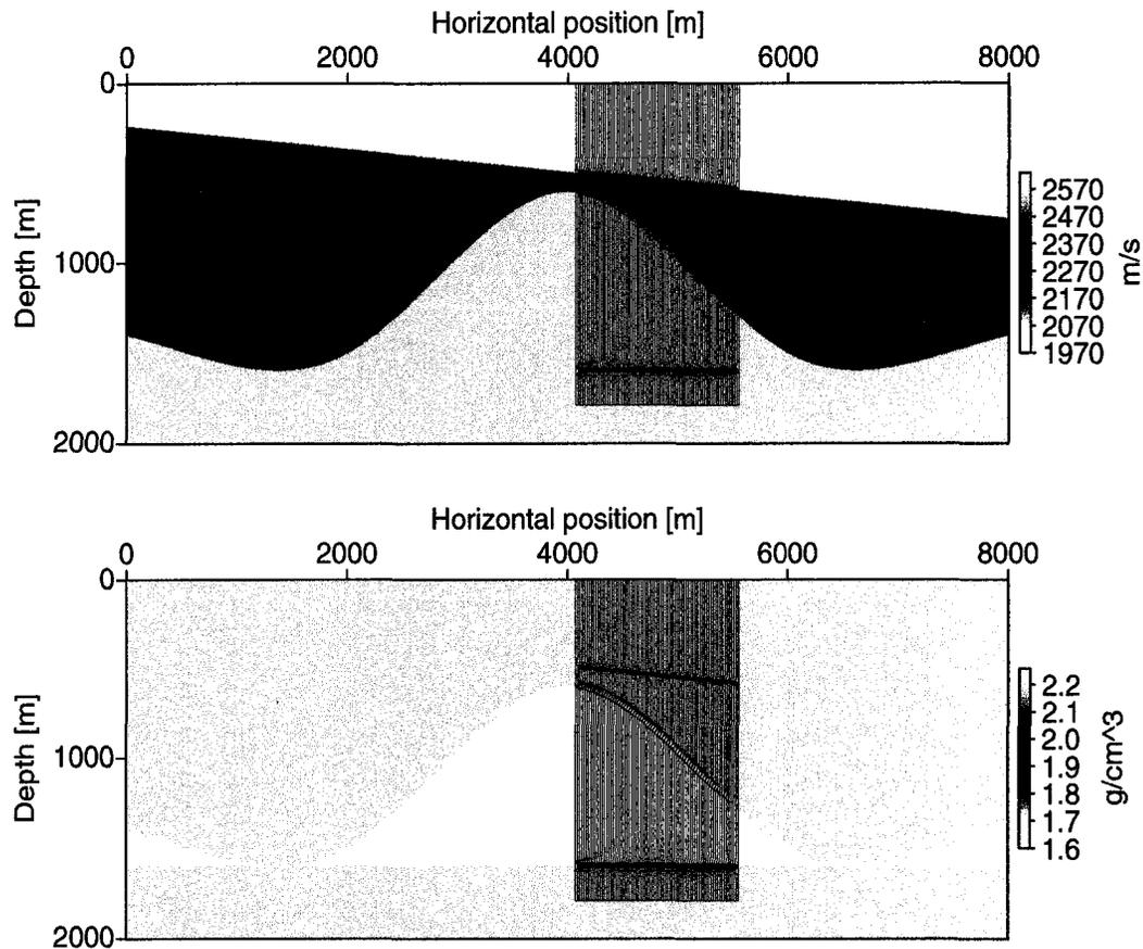
Figure 3.35: Velocity (top) and density model (bottom) with a slightly dipping, a moderately curved and dipping, and a flat reflector. The flat reference reflector is represented by a density change only. The migrated and stacked sections are shown as overlays.
