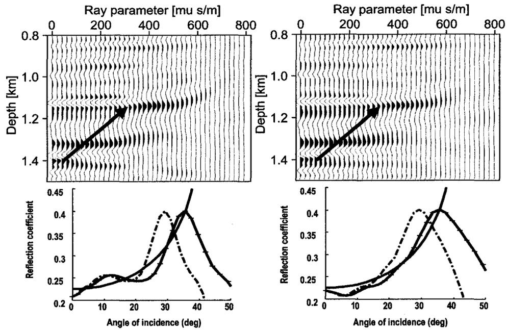
Figure 3.44: Left: Blow-up of the least-squares migrated target reflector CIG (4 iterations) and the picked AVA curve (complete wavefield data). The dot-dashed line is the AVA without dip correction. Right: Blow-up of the least-squares migrated target reflector CIG (12 iterations) and the corresponding AVA (incomplete wavefield data).
