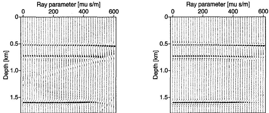
Figure 3.36: Left: Migrated CIG at CMP location 4600 m (see Figure 3.35). Finite aperture effects and offset aliasing cause spurious energy in the CIG. Right: Least-squares CIG (6 iterations) at CMP location 4600 m. Most of the spurious energy has been cleaned up. The picked AVA for the second and the third reflector are shown in Figure 3.37.
