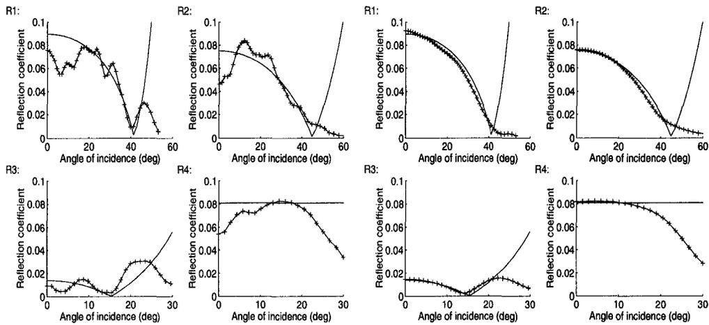
Figure 3.28: Left (R1-R4): AVA picked on the migrated CIG in Figure 3.26 (left). 50% of the data were randomly set to zero prior to migration (see also Figure 3.22). Right (R1-R4): The same picks based on the least-squares migrated CIG (14 iterations) in Figure 3.26 (right).
