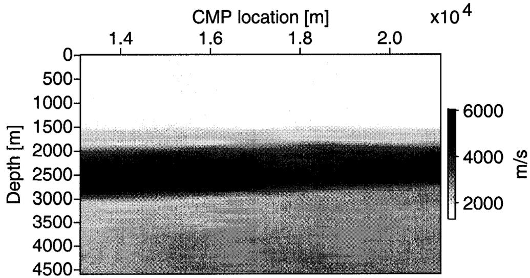
Figure 4.3: The migration velocity field obtained by spatial interpolation of the 1-D least-squares 'Dix inversion' result and time to depth conversion.
