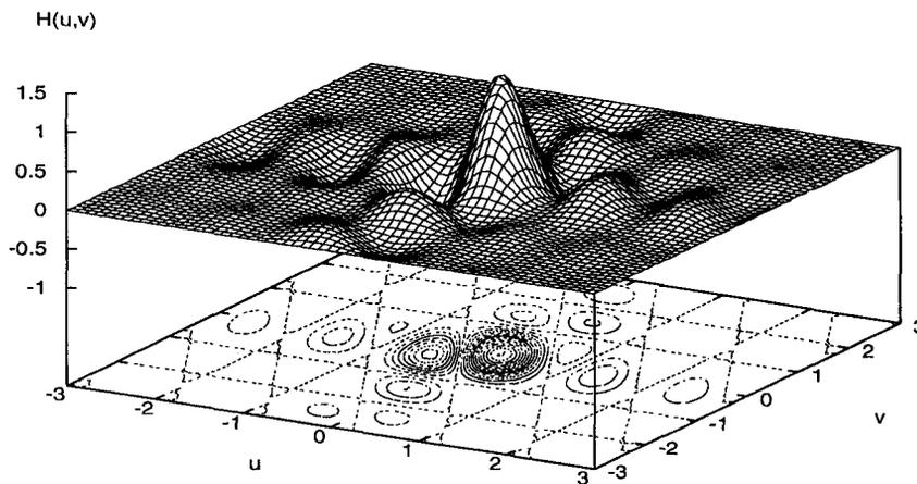
Figure 5.4: The Hartley transform of the 2-D boxcar function in Figure 5.1. The Hartley transform exhibits no symmetry and codes phase and amplitude information in a single real-valued function.
