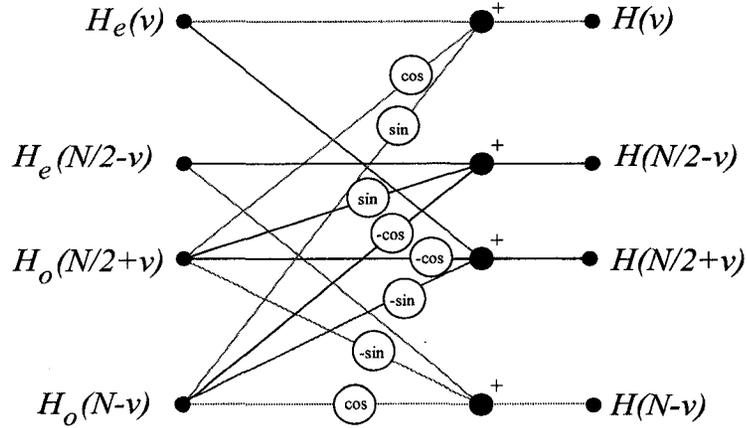
Figure 5.5: The ‘Hartley butterfly’ according to equation (5.1.8). The sine and cosine factors are evaluated at  $\frac{2\pi}{N}\nu$ , where  $N$  is the length of the discrete sequence (after Sorensen et al. (1985)).
