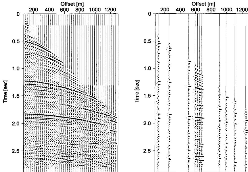
Figure 3.41: Left: CMP data at location 7500 m of the Marmousi model. Notice that the first live trace is at (half) offset 100 m. Right: The CMP after removing 70% of the live traces.
