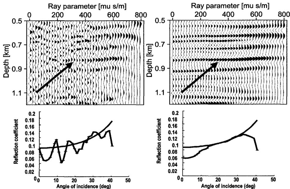
Figure 3.42: Left: Blow-up of the migrated target reflector and the picked AVA curve (incomplete wavefield data). Right: Blow-up of the least-squares migrated target reflector CIG (12 iterations) and the corresponding AVA (incomplete wavefield data).
