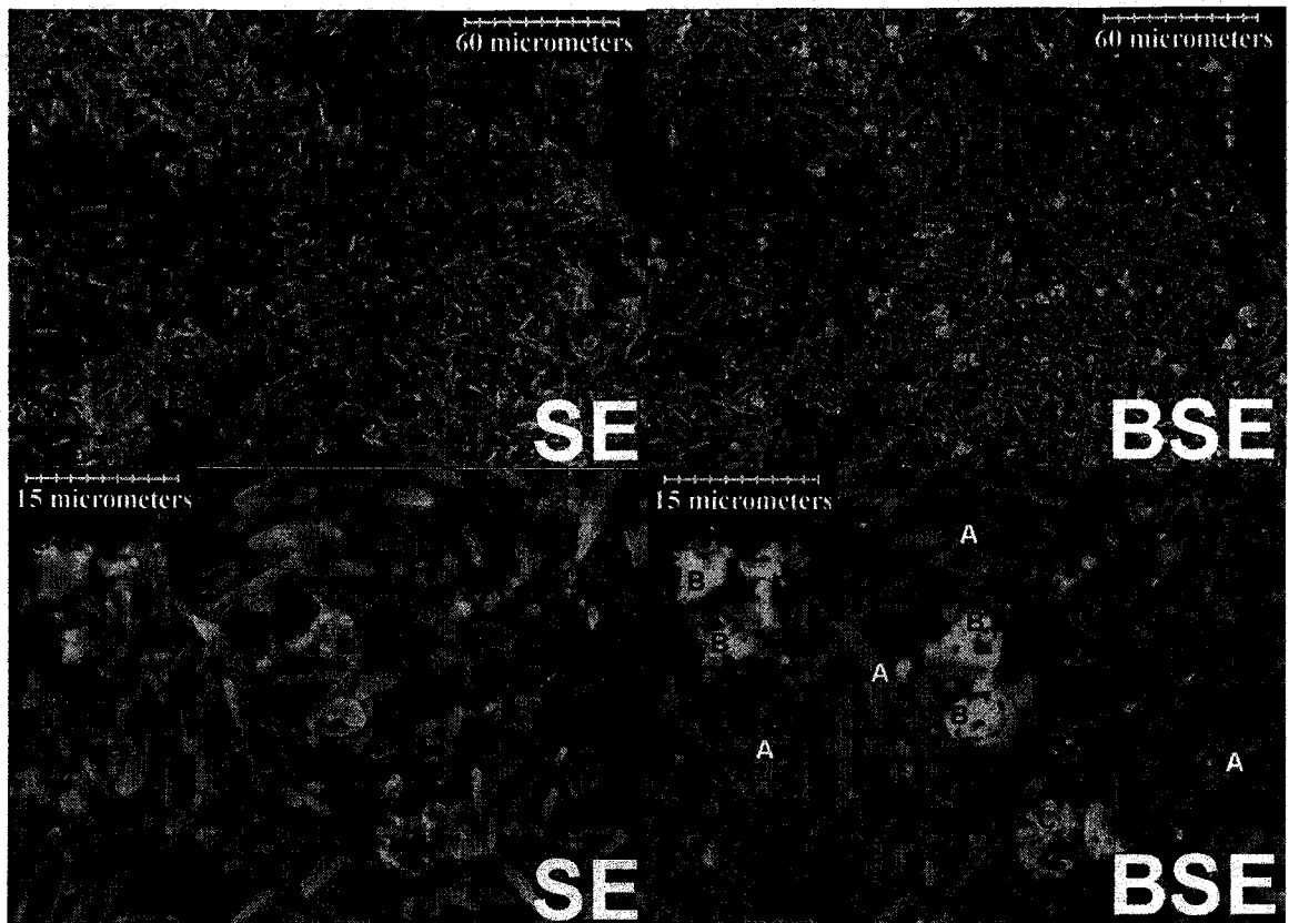
Figure 105 Secondary Electron (SE) and Backscattered Electron (BSE) Images of EAF Dust after Roasting at 1000°C with 16% Coal and Leaching with 200 g/L H 2 SO 4 (Sample C)
