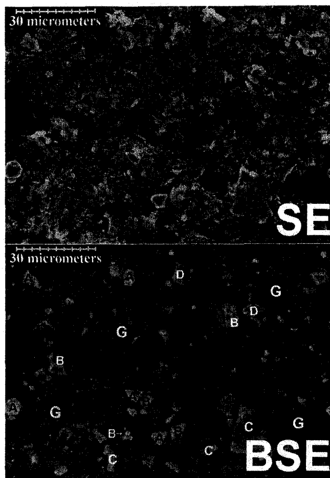
Figure 92 Secondary Electron (SE) and Backscattered Electron (BSE) Images of EAF Dust after Roasting at 1000°C with 90% \text{Na}_2\text{CO}_3 and 3.7% \text{CaCO}_3 and Leaching with 200 g/L \text{H}_2\text{SO}_4 (Sample D)
