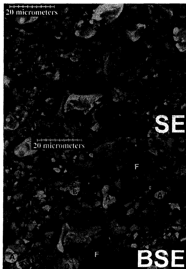
Figure 89 Secondary Electron (SE) and Backscattered Electron (BSE) Images of EAF Dust after Roasting at 1000^\circ\text{C} with 50% \text{Na}_2\text{CO}_3 and 3.7% \text{CaCO}_3 (Sample C)
