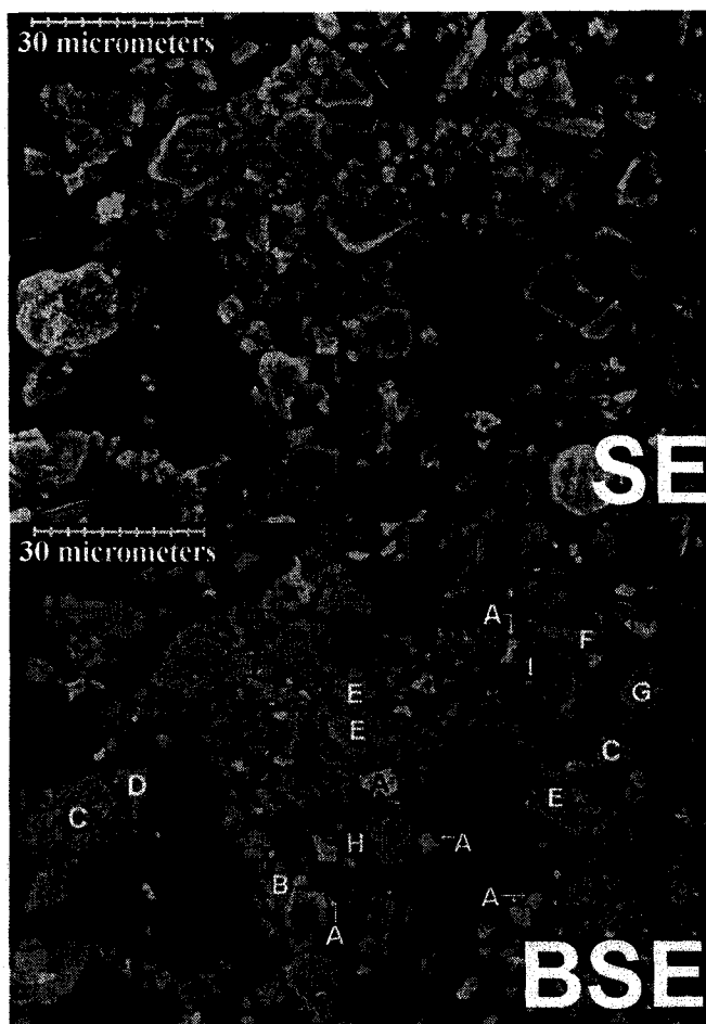
Figure 78 Secondary Electron (SE) and Backscattered Electron (BSE) Images of EAF Dust after Roasting at 950°C with 40% \text{Na}_2\text{CO}_3 (Sample D)
