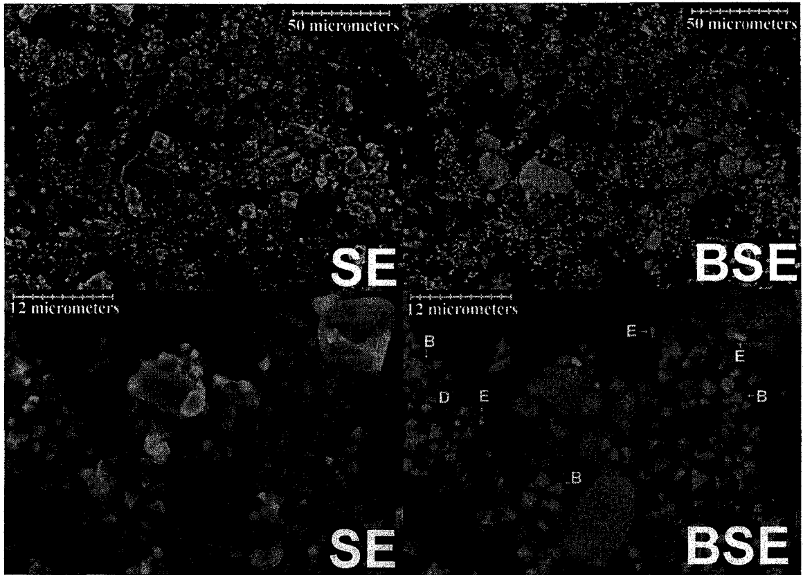
Figure 80 Secondary Electron (SE) and Backscattered Electron (BSE) Images of EAF Dust after Roasting at 950^\circ\text{C} with 80% \text{Na}_2\text{CO}_3 and Leaching with Hot Water (Sample E)
