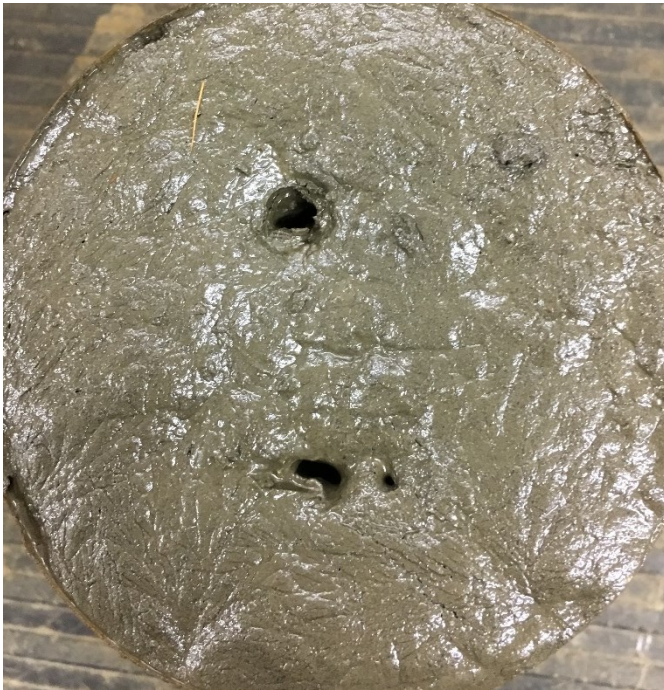
Figure 6-3: Sample BG3 Following Completion of Freezing
