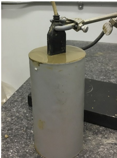
Figure 3-4: Example of a TDR calibration test
