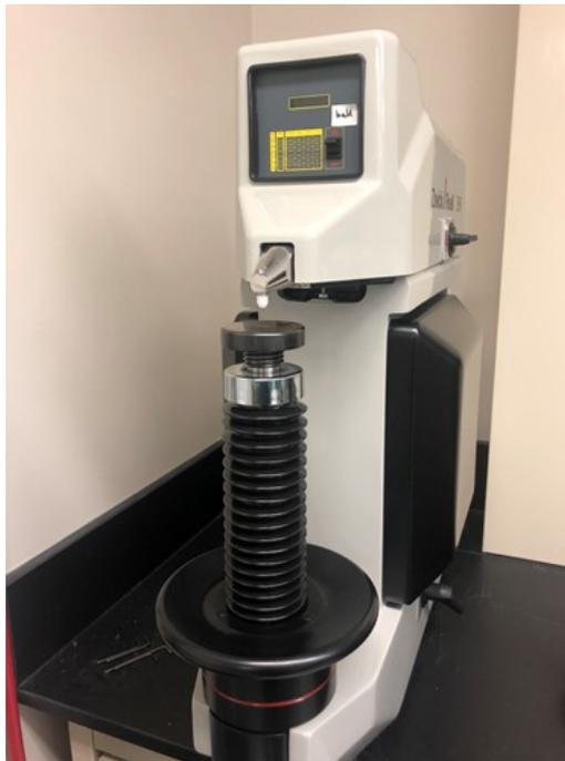
Figure 2.2 ZHR Rockwell hardness tester
