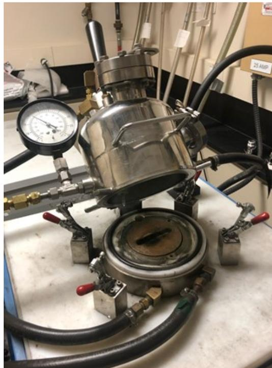
Figure 2.1 Arc furnace used to make samples for the present study
