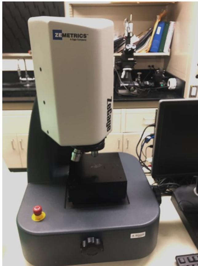
Figure 2.4 3D Optical Surface Profiler (ZeGage, ZygoCorp)
