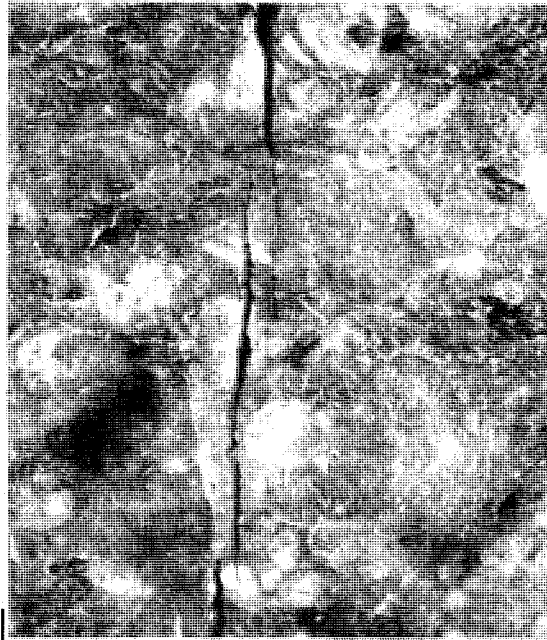
Figure 4.1 : An extension fracture generated in uniaxial compression in granite. The fracture is parallel to the direction of loading and the grain size is approximately 3 mm. Note the open irregular geometry of the fracture.
