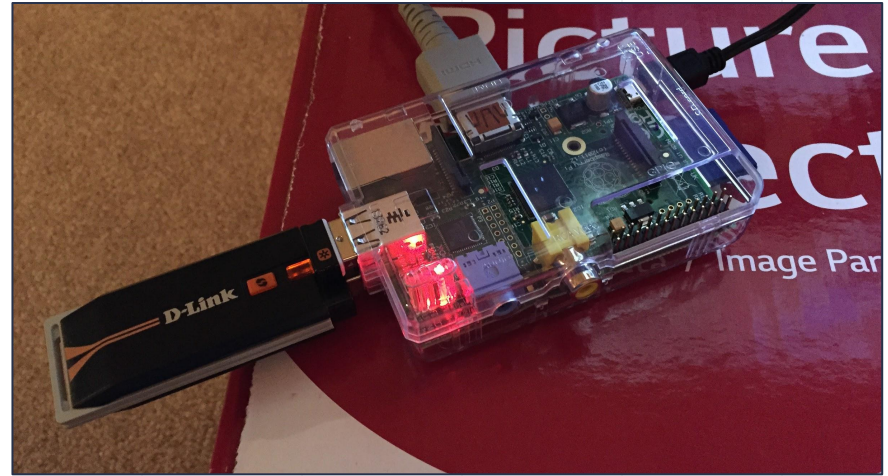
Homemade TV media centre: Raspberry Pi model B+ running OpenElec
