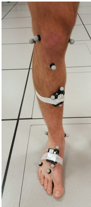
Fig. 8. Illustration of the Technical Validation set-up: Anatomical (applied to bony landmarks) and technical (applied to sensors boxes) markers, as well as the two IMUs, affixed on the right foot (along the second metatarsal) and leg (medial upper shank) of the participant, are represented. Among the anatomical markers, only the second and fifth metatarsal and calcaneal tuberosity markers were used for this study. No marker was present in the Clinical Research Application study.
