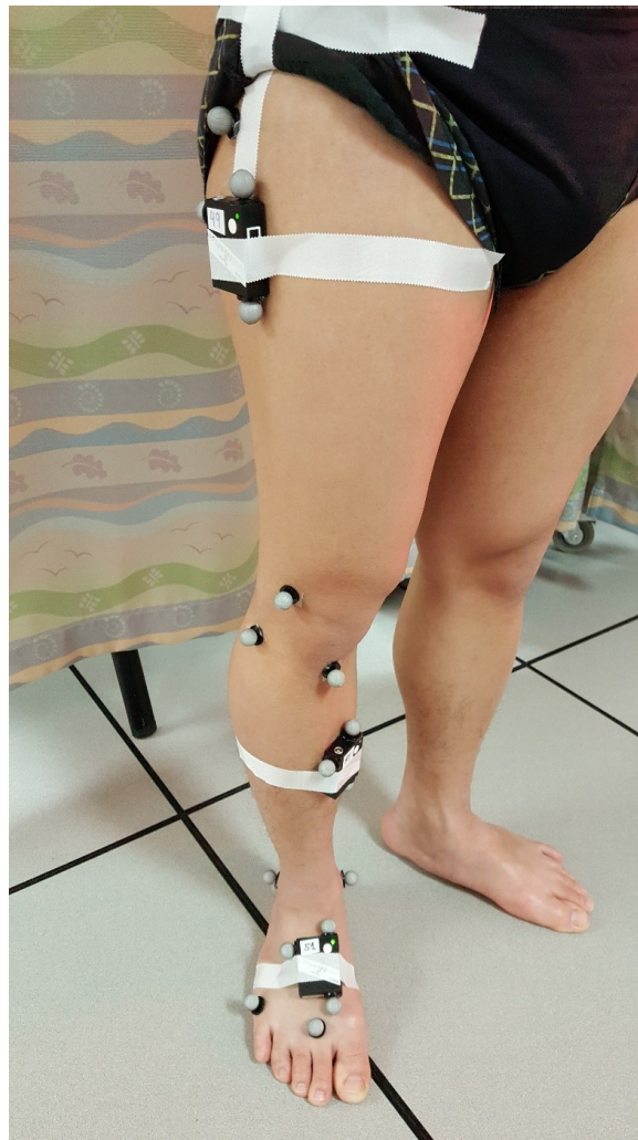
Fig. 4. Anatomical and sensor-box reflective markers, and the 3 IMUs, placed on the right thigh, shank, and foot of the participant for validation of the 3D knee and ankle angles estimated by the IMUs against the motion-capture system. Anatomical markers were removed after a 1-min upright standing still period was recorded with the cameras.
