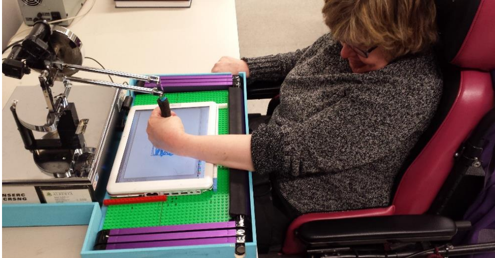
Figure 1. The individual with CP operating the robotic system, equipped with the virtual assistance, by holding the robotic end-effector
