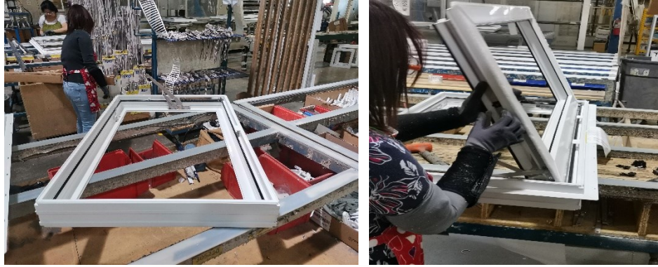
Figure 3-7. Frame hardware installation station
