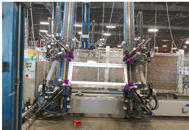
Figure 3-5. Profile welding station
