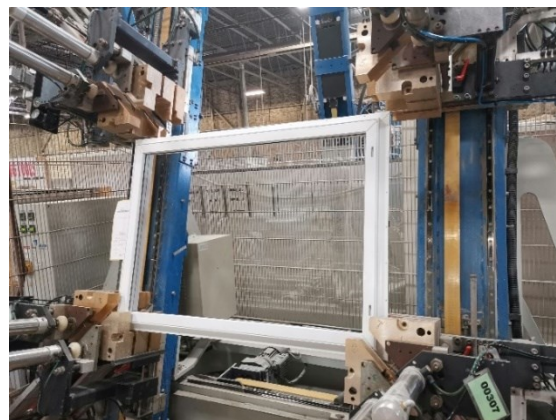
Figure 3-10. PVC welding station
