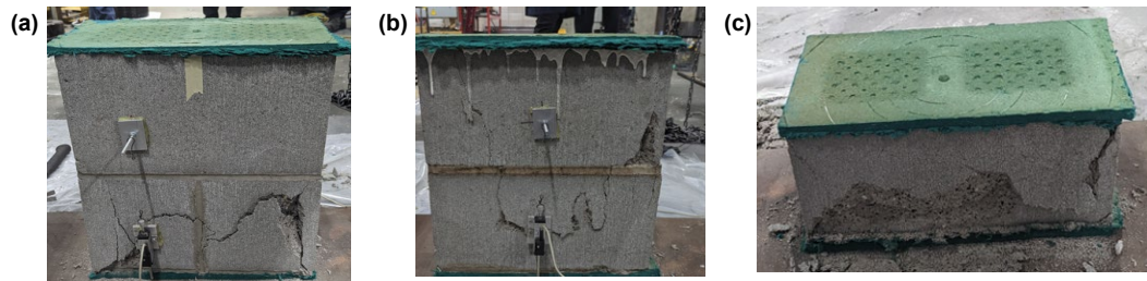
Figure A.3: Auxiliary concrete masonry unit specimen testing of (a) two course ungrouted, (b) two course grouted, (c) one block from Elsayed, Alonzo and Gonzalez experimental work
