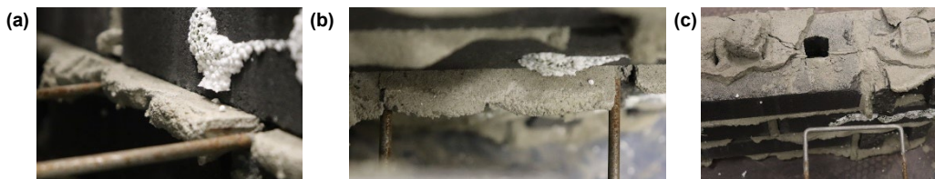
Figure C.9: T-R.CN-1 after testing of (a) embedding failure, (b) top view of embedding failure, (c) top view after connector removal
