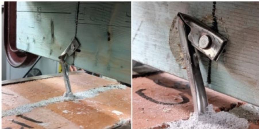
Figure 2.11: Primary failure mode in compression from Muhit et al. (2022)
