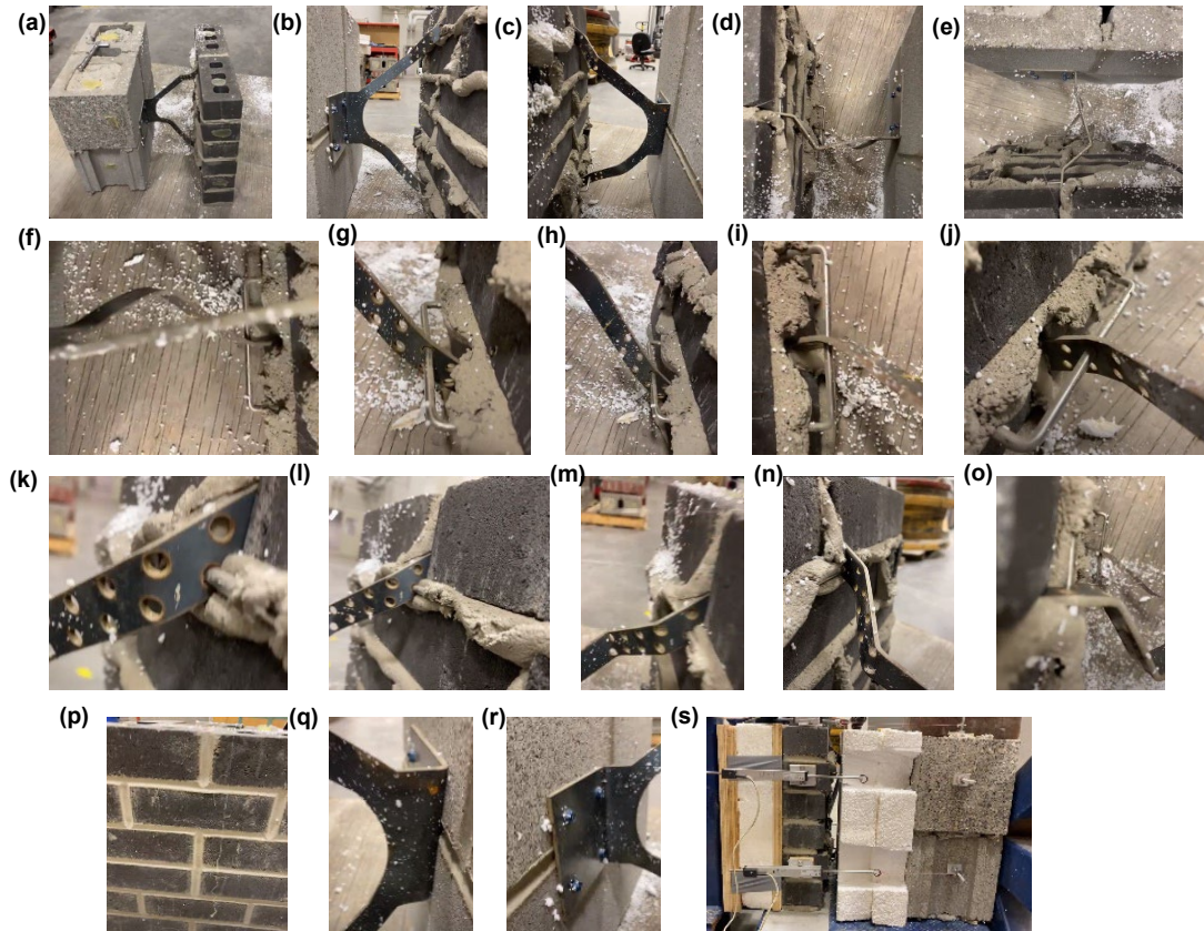
Figure C.56: C-IN.CN-3 after testing of (a) side view, (b) side view 2, (c) side view 3, (d) top view, (e) top view 2, (f) top view with bottom connector leg focus, (g) bottom connector leg side view, (h) bottom connector leg side view 2, (i) bottom connector leg top view, (j) bottom connector leg top view 2, (k) top connector leg side view, (l) top connector leg side view 2, (m) top connector leg side view 3, (n) top connector leg side view 4, (o) top connector leg top view, (p) outside face of brick veneer condition, (q) CMU connector interface view, (r) CMU connector Tapcon fastener interface view 2, (s) specimen view during testing
