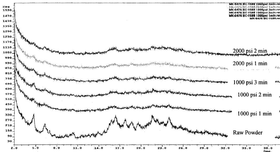
Figure 3-18 Montelukast sodium: X-ray powder diffraction pattern
