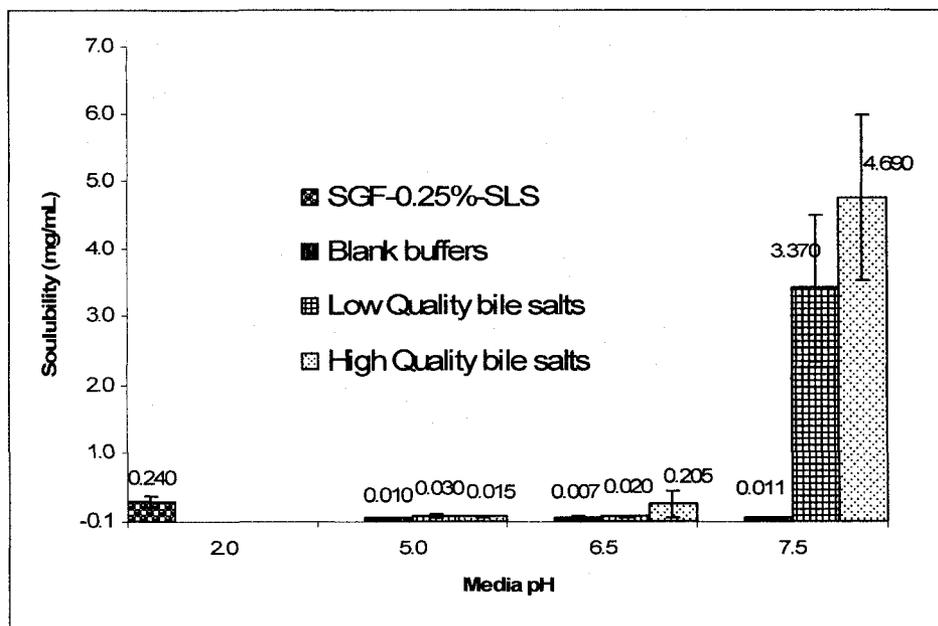
Figure 3-17 Montelukast sodium: solubility in SGF with 0.25% SLS, blank and biorelevant media containing High and Low quality bile salts and lecithin.
