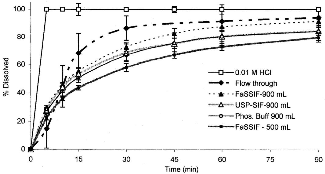
Figure 3-9 Etoricoxib: Comparison of dissolution profiles in the USP Apparatus 2 and the Flow through cell.
