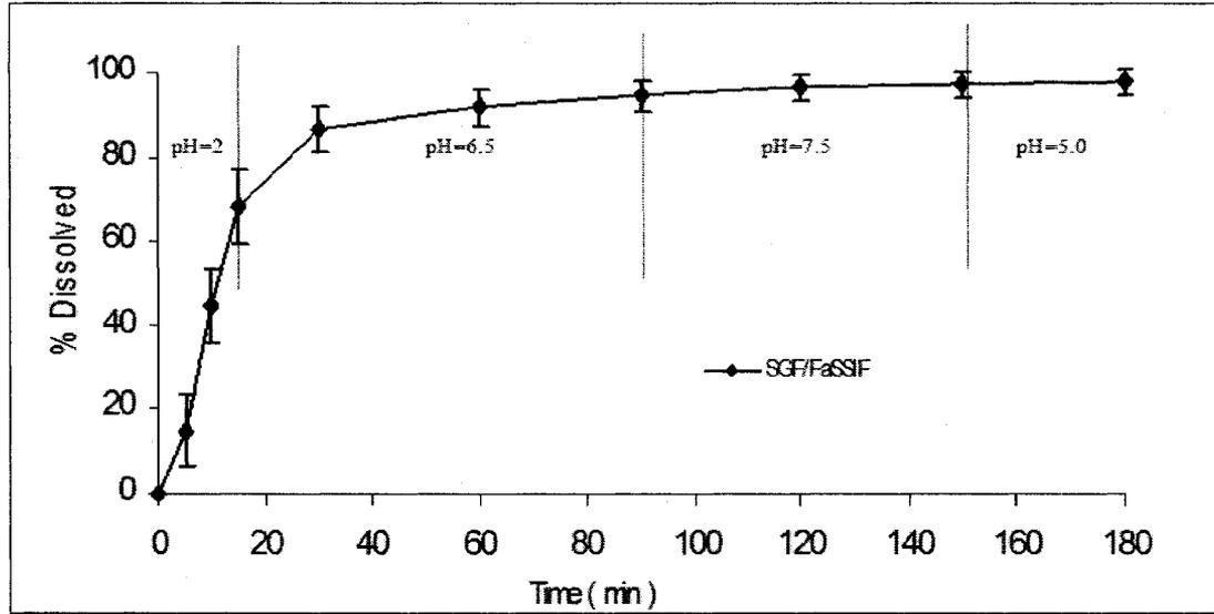
Figure 3-8 Etoricoxib: Dissolution profile in the flow-through cells following the dynamic pH change protocol (n=6)
