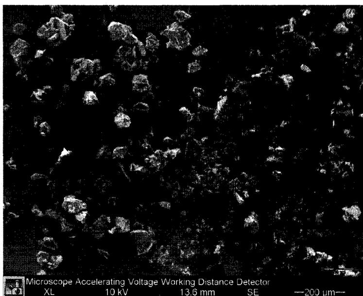
**Figure 3-6 Etoricoxib: Scanning electron micrograph (SEM) of the API powder**
