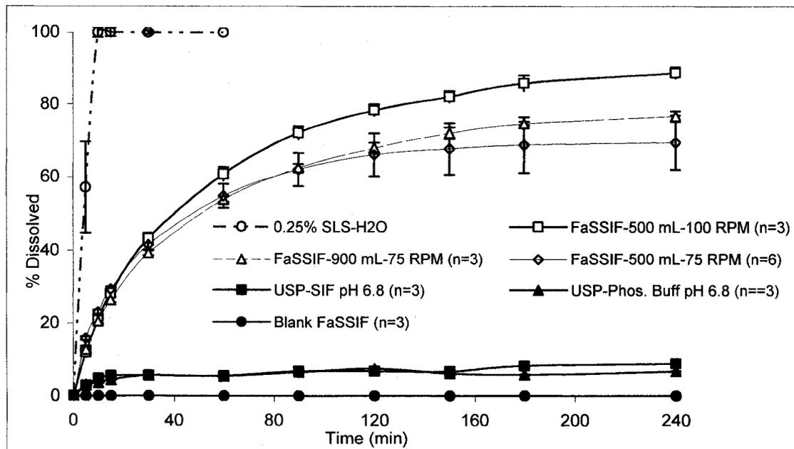
Figure 3-22 Montelukast sodium: Dissolution profiles in various media using the USP apparatus-2
