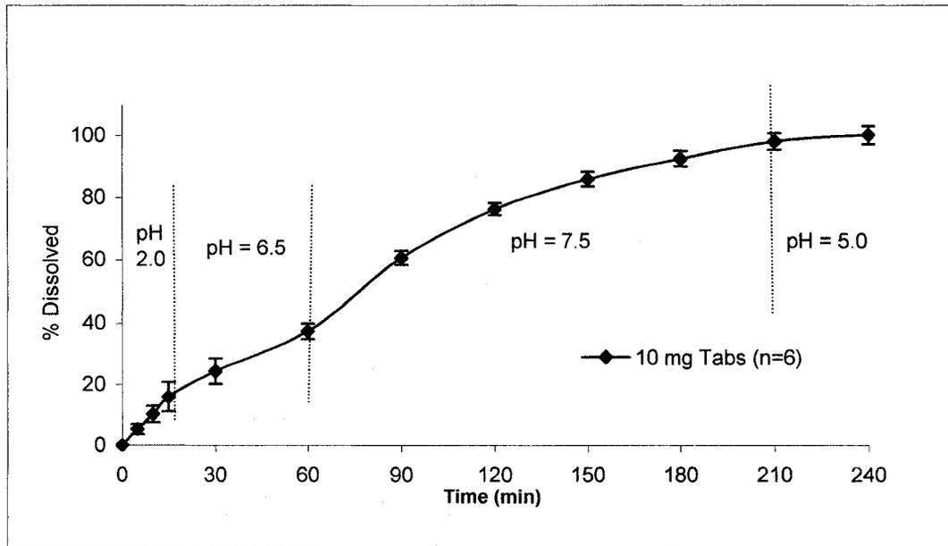
Figure 3-21 Montelukast sodium: Dissolution profile in the flow-through cells following the dynamic pH change protocol (n=6)
