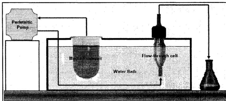
**Figure 2-2 Set-up of Flow through cell Dissolution Tester**
