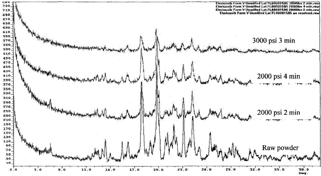
Figure 3-2 Etoricoxib: X-ray diffraction pattern of the API
