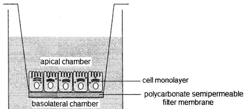
**Figure 2-3 Schematic drawing showing cell monolayer on a transwell insert plate**
