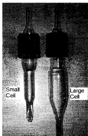
**Figure 2-1 The Small and Large flow through cells**
