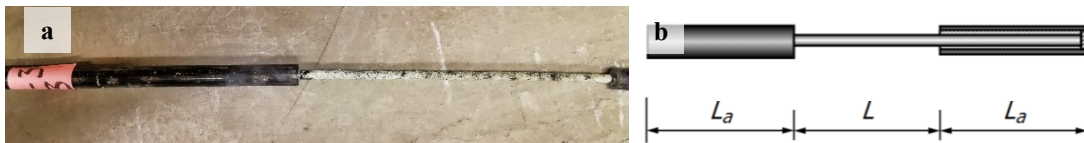
Figure A1.2: Anchored test specimen (a) photo (b) figure (ASTM International, 2016).
