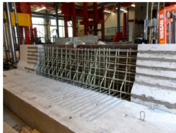
Figure 2.15: NSM technique showing NSM groove layout and photograph of NSM reinforcement (El-Salakawy et al. 2014).
