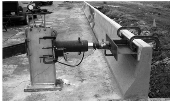
Figure 2.9: Test setup for static load testing (Alberson et al. 2004).
