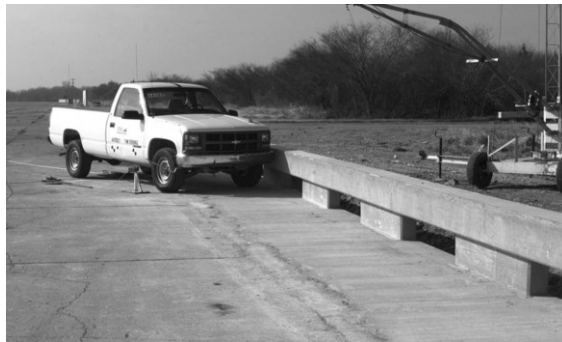
Figure 2.13: Open post-railing reinforced with GFRP and test vehicle (Buth et al. 2003).
