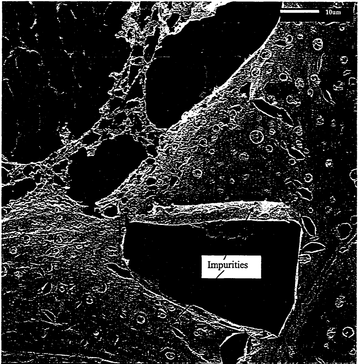
Figure 4.66: 1000x magnification scanning electron microscope image of a fractured ice specimen produced from spray freezing of pulp mill effluent at -10\text{ }^{\circ}\text{C} and stored at the spray temperature for 2 days, showing impurities inside a pore.
