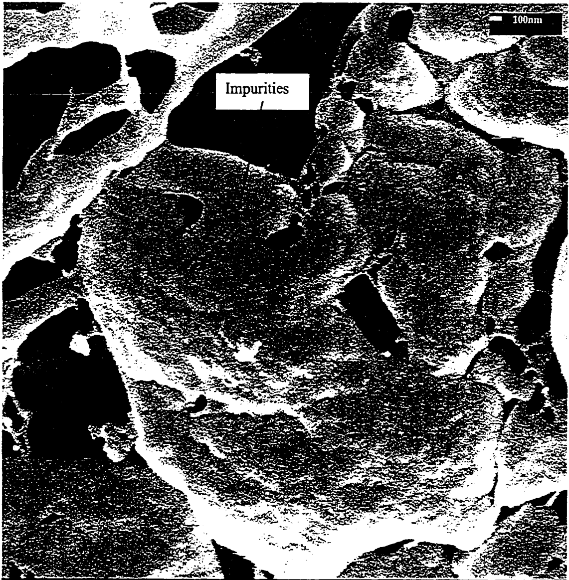
Figure 4.73: 20000x magnification scanning electron microscope image of a fractured ice specimen produced from spray freezing of pulp mill effluent at -10\text{ }^{\circ}\text{C} and stored at the spray temperature for 14 days, showing impurities inside a pore.
