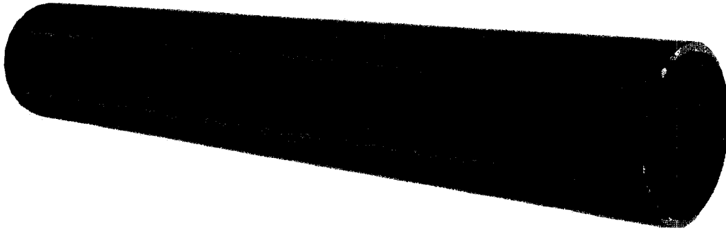
Figure 7.4: Prospective view of one LUCID module in the GEANT4 simulation. The readout structures are not shown.
