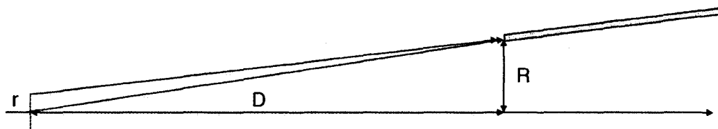
Figure A.2: Effect of beam size on LUCID acceptance. The horizontal line is the Z axis.
