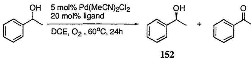
**Scheme 3.17** Enantioselective palladium (II)-catalyzed aerobic alcohol oxidation
