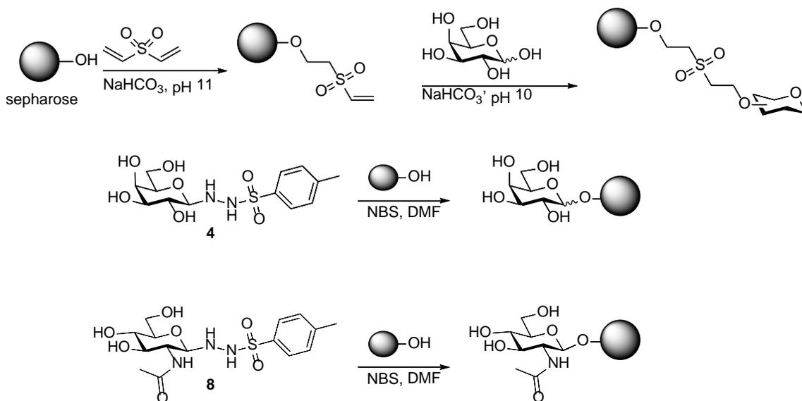
**Figure 3. Immobilization of galactose to Sepharose using DVS and GSH chemistries.**
