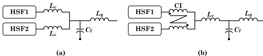
Figure 6.17. Illustration of two filter architectures, (a) modular architecture and (b) coupled architecture.
