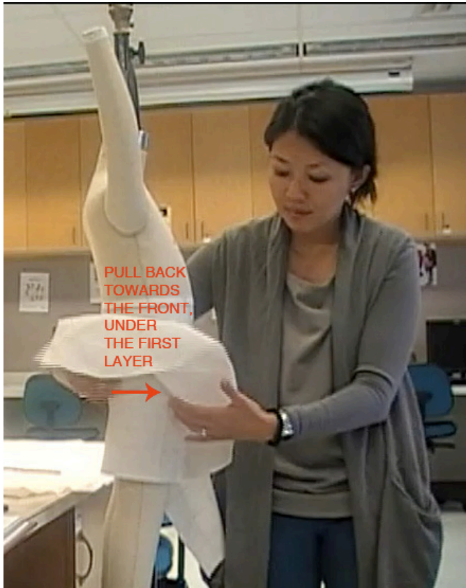
Figure 45e: Step Five - Pull the end towards the front again under the first layer.
