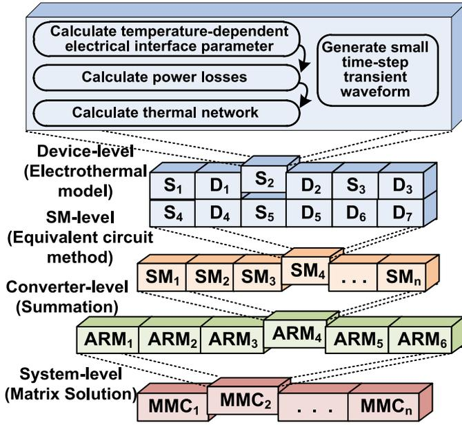
Fig. 6. Illustration of hierarchical MMC modeling scheme.
