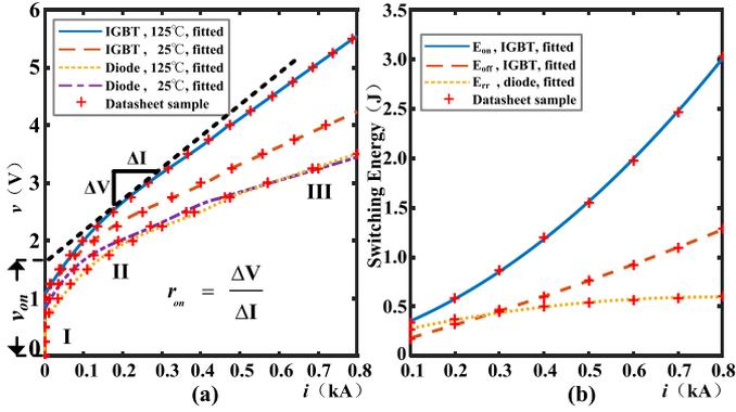
Fig. 4. Datasheet sample and fitted curves of the Infineon FZ400R33KL2C\_B5 IGBT and diode characteristics. (a) Output characteristics of IGBT and diode at 125 °C and 25 °C. (b) switching energy losses of IGBT turn-on, IGBT turn-off and diode reverse recovery processes at 125 °C.
