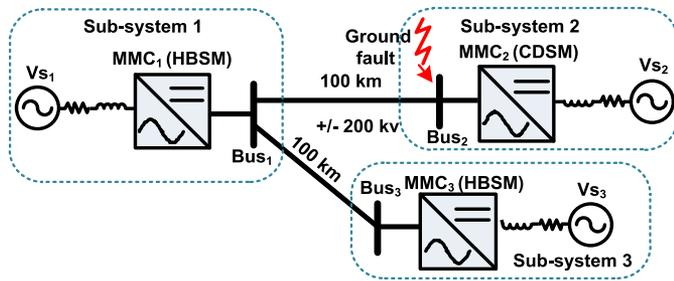
Fig. 8. Circuit topology of MMC-based three-terminal MTDC system.
