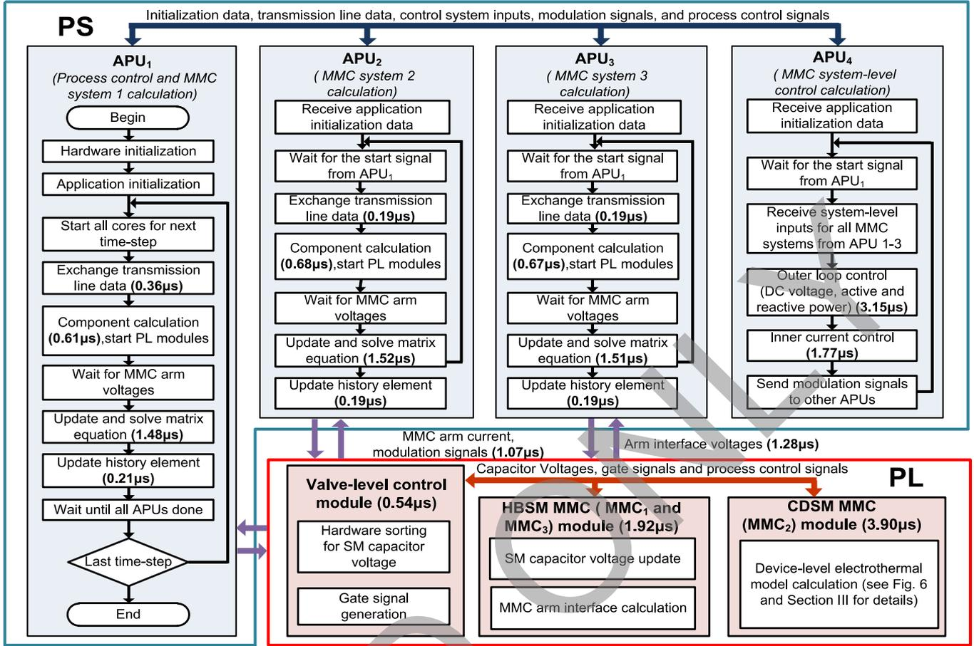
Fig. 9. Design partition of the MTDC system on the MPSoC device (latencies are shown in parentheses).
