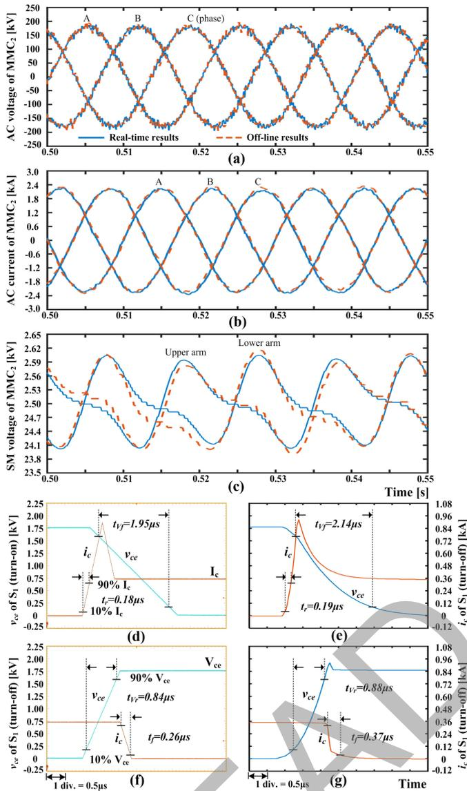
Fig. 10. Steady state results. (a) AC voltages. (b) AC currents. (c) SM voltages. (d) (e) Turn-on switching transients of  $S_1$ . (f) (g) turn-off switching transients of  $S_1$ . (In (a) (b) (c), the solid lines are real-time results, and the dashed lines are offline PSCAD/EMTDC results. (d) (f) are real-time results, and (e) (g) are offline SaberRD results.)
