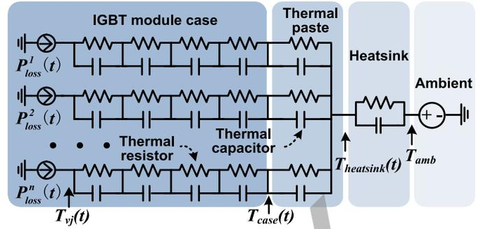
Fig. 5. Equivalent circuit for IGBT module thermal network.
