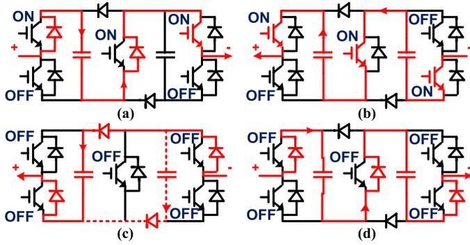
Fig. 2. CDSM operation demonstration with active routes in color red. (a) Normal operation with positive arm current. (b) Normal operation with negative arm current. (c) Protection mode with negative arm current. (d) Protection mode with positive arm current.
