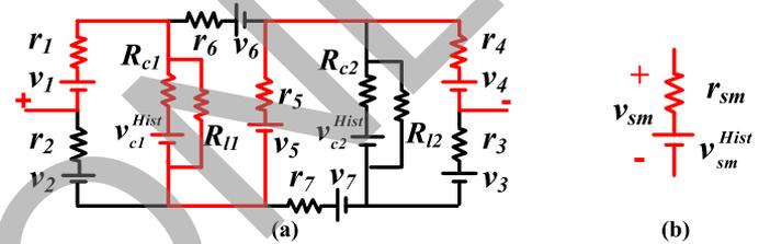
Fig. 3. CDSM models. (a) Complete circuit model with active route. (b) Simplified SM interface model.
