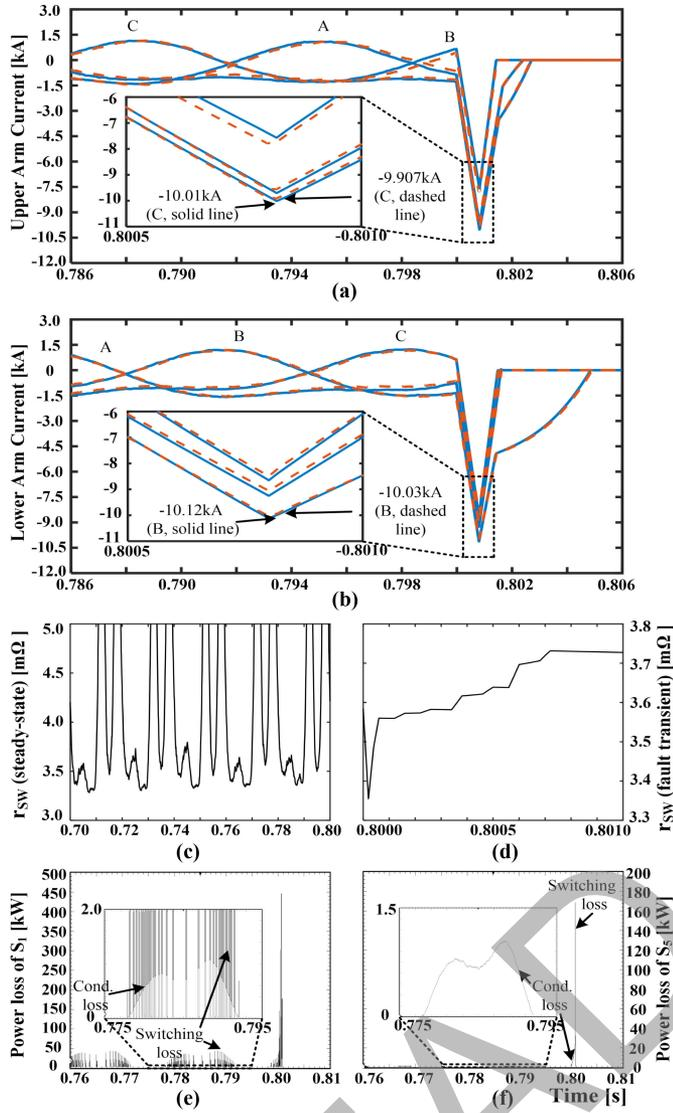
Fig. 12. Fault transient results. (a) Upper arm currents. (b) Lower arm currents. (c) IGBT resistance  $r_{sw}$  of  $S_1$  during steady-state. (d) IGBT resistance  $r_{sw}$  of  $S_1$  during fault transient. (e) Power loss of  $S_1$ . (f) Power loss of  $S_5$ . (In (a) (b), the solid lines are real-time results, and the dashed lines are offline PSCAD/EMTDC results. (c)–(f) are real-time results.)
