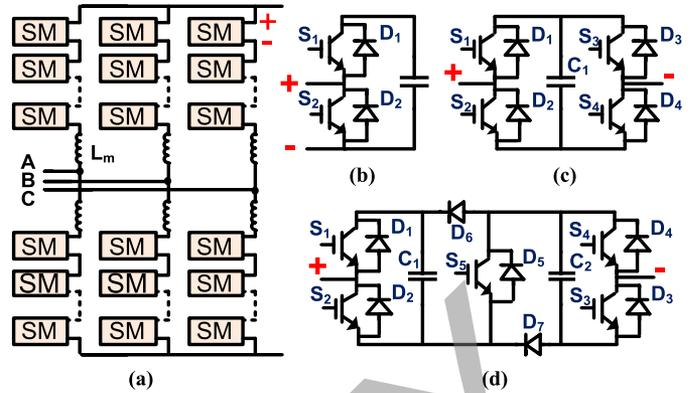
Fig. 1. MMC and SM topologies. (a) Modular multi-level converter. (b) Half-bridge submodule. (c) Full-bridge submodule. (d) Clamp double submodule.
