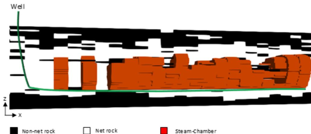
Figure 5.8: Steam-chamber of well located in second quadrant and level 7.
