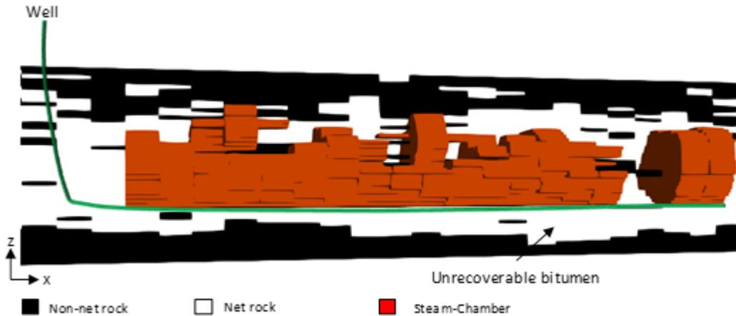
Figure 5.9: Steam-chamber of well located in second quadrant and level 10. Note the large amount of unrecoverable bitumen below the producer well.
