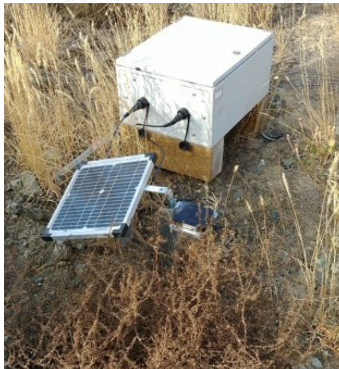
Figure 4-3: 10-Mile Slide GPS unit final setup (Rodriguez 2017)
