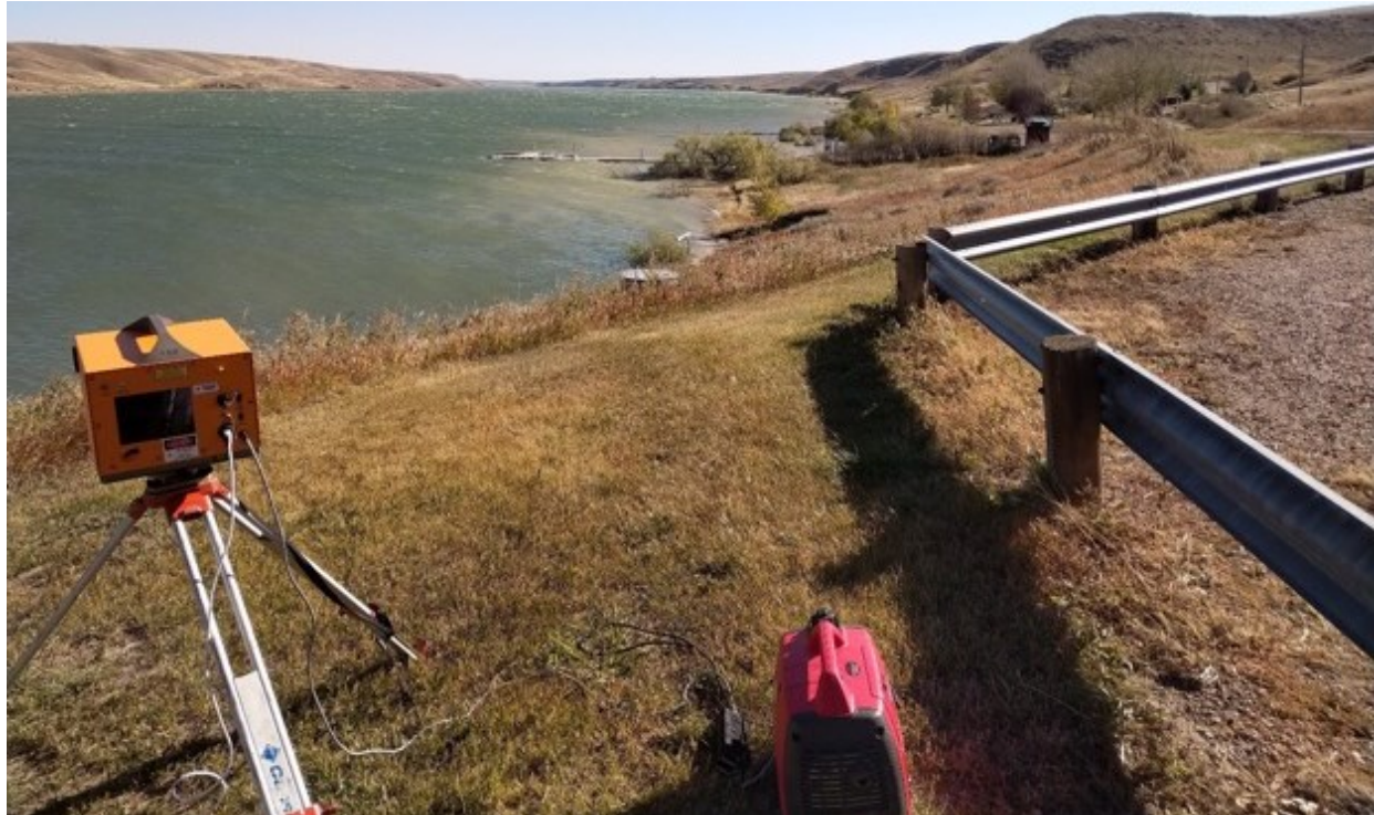
Figure 5-1: ILRIS-LR LiDAR scanner used on Chin Coulee (Location 1)
