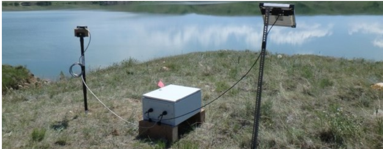
Figure 4-4: Solar panel, GPS unit, and battery box setup on Chin Coulee (Hong 2018)
