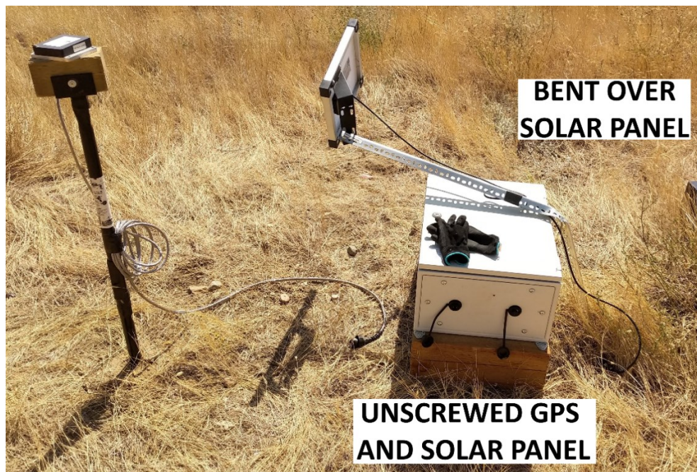
Figure 4-13: Vandalism to Geocube on Chin Coulee. GPS and solar panel unscrewed and damaged
