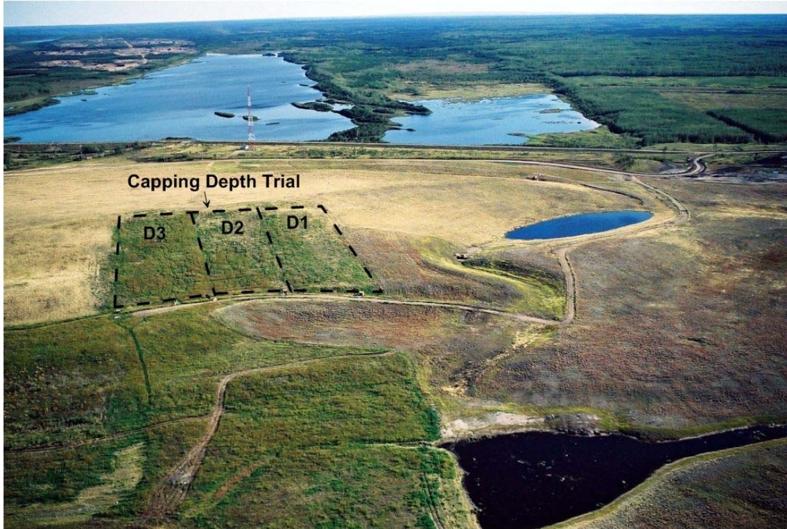
Figure 2-3. North side of SBH after reclamation, featuring capping trial area (2001).
