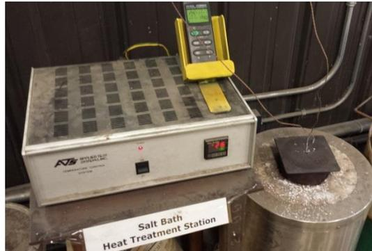
Figure 3.10 Salt bath furnace attached with a thermocouple.
