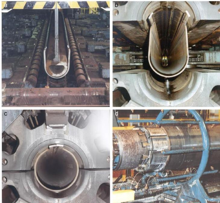
Figure 2.9 Photographs of (a) U-press, (b)-(c) O-press and (d) expansion [1].
