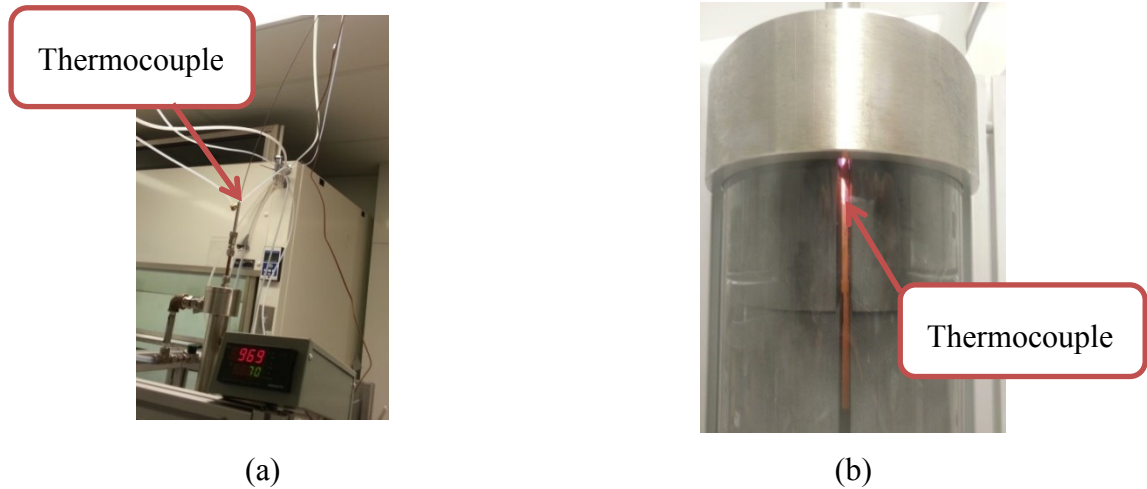
Figure 2-20 -(a) centerline temperature measurements experiment (b) thermocouple inside the flame
