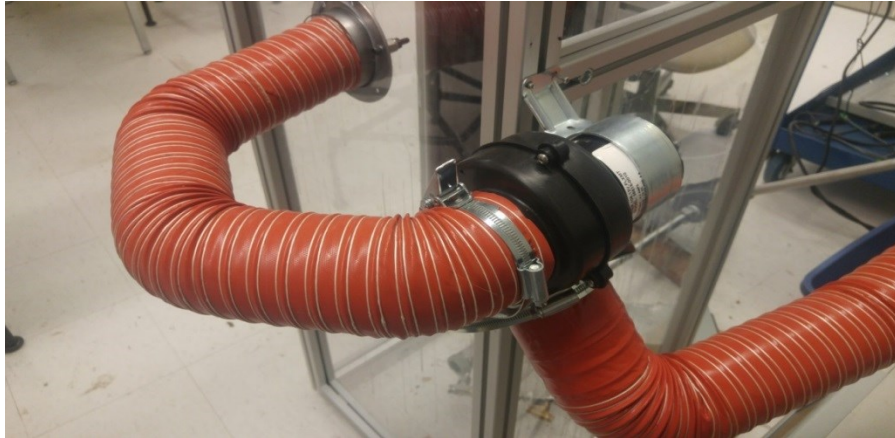
Figure 2-13 - Actual image of the vacuum pump and duct hose
