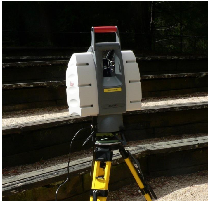
Figure 2-4: A Leica HDS-3000 Laser Scanner (Courtesy: David Monniaux)
