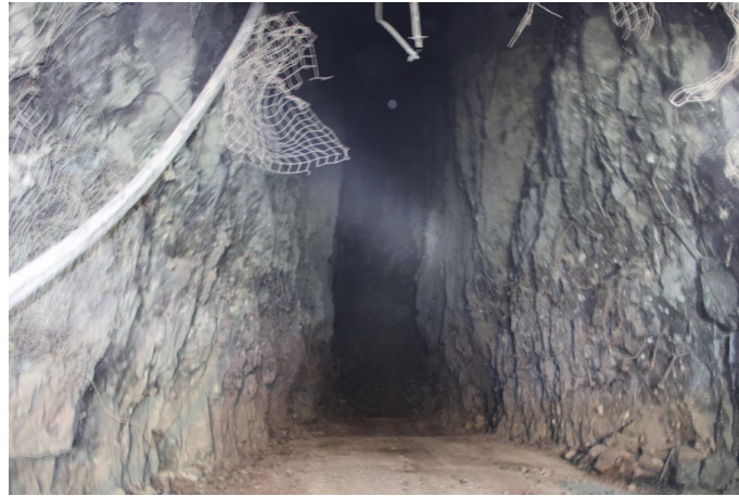
Figure 4. 13 View of typical open stope at the analyzed underground diamond mine (Photo by authors)
