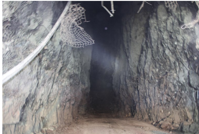
Figure 4. 7 View of typical open stope at the analyzed underground diamond mine (Photo by authors)
