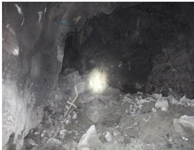
Figure 1. 1 A rock burst case at a diamond mine in Canada (photo taken by author)
