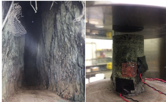
Figure 5. 8 A typical mining stope in kimberlite and a kimberlite sample for UCS test
