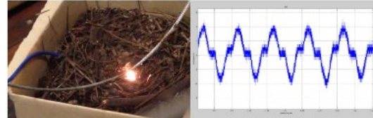
Figure A.4 Typical soil arc and waveform
