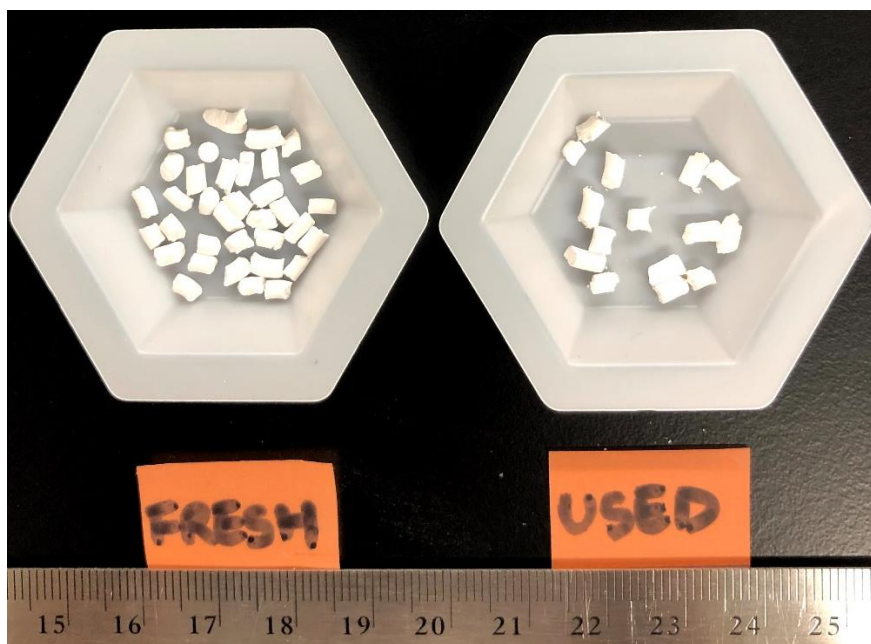
Figure 7.12: The appearance of the fresh CALF-20 and the used sample
