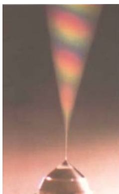
Figure 1.2 Example of a stationary Taylor cone, adapted from Ref 58.
