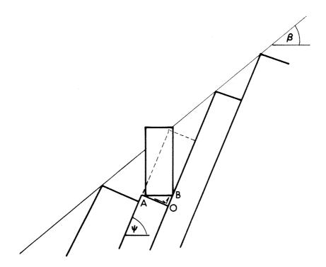
Figure 1. Toppling by sliding on 2 surfaces
