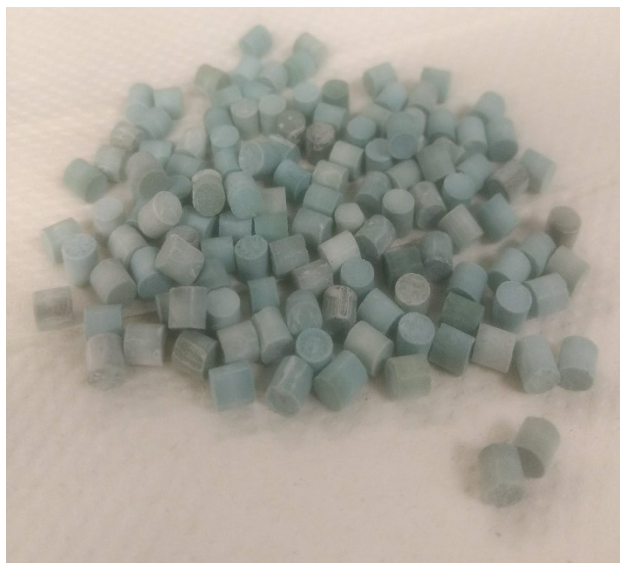
Figure 3.1 Ni/ \gamma -Al 2 O 3 catalyst pellets used for hydrogenation reactions
