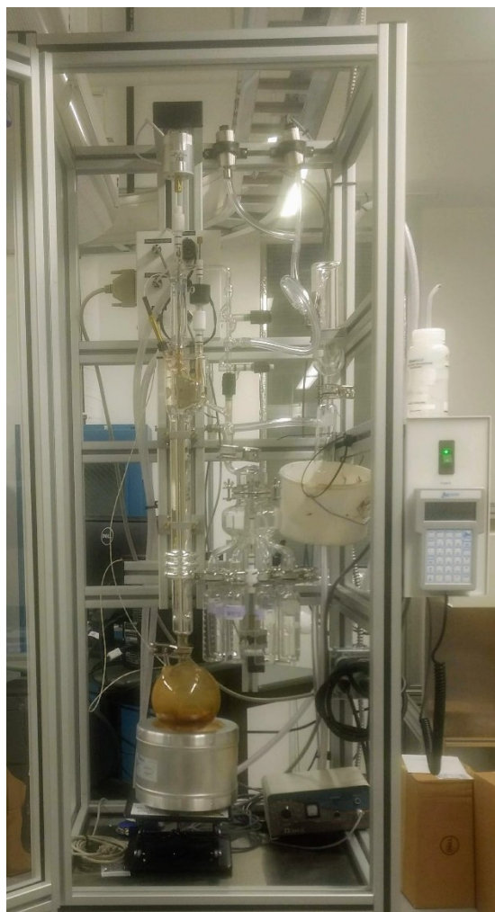
Figure 4.1 BR M690 Distillation system used for fractionation of cracked naphtha
