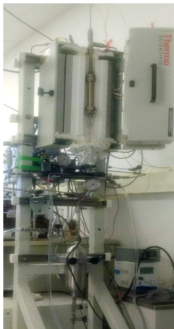
Figure 3.3 Images of the continuous flow reactor designed for hydrogenation reactions
