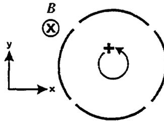
**Figure 1.2** Illustration of the cyclotron motion of a positive ion in the presence of constant magnetic field ( $B$ ).
