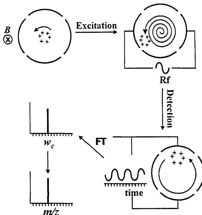
**Figure 1.3** Illustration how a mass spectrum is obtained from the ICR motion.
