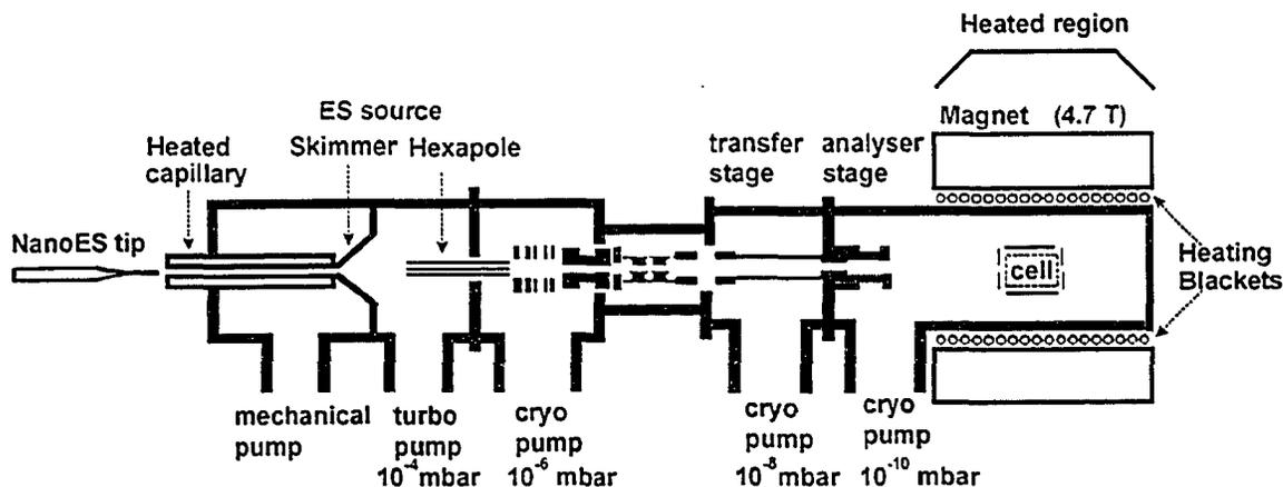
**Figure 1.4** NanoES-FT-ICR/MS instrument diagram.
