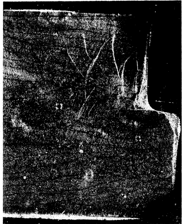
Fig. 20. Edge structures in specimen H4. Full height (one inch) shown. Crossed polars
