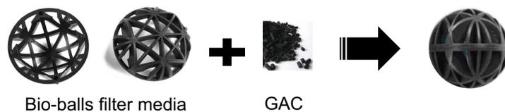
**Fig. 7.1. The top-GAC bio-balls.**
