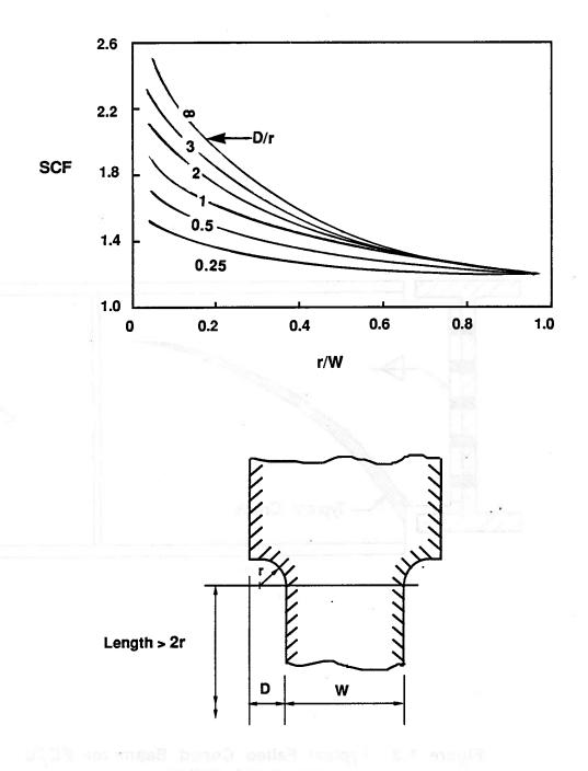
Figure 1.4 Fatigue Stress Concentration Factor for Re-entrant Corners
