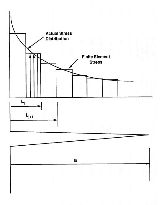
Figure 5.1 Finite Element Discretization for  $F_{\rm G}$
