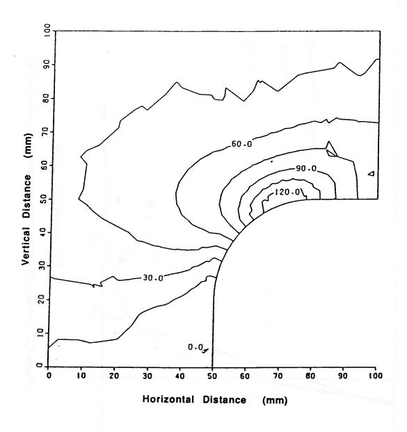
Figure 4.7 Stress Contour for 30 mm Cope Radius
