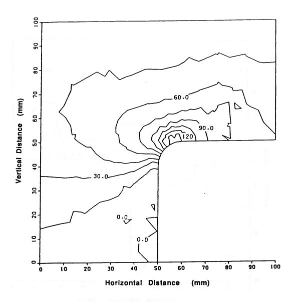
Figure 4.5 Stress Contour for 10 mm Cope Radius
