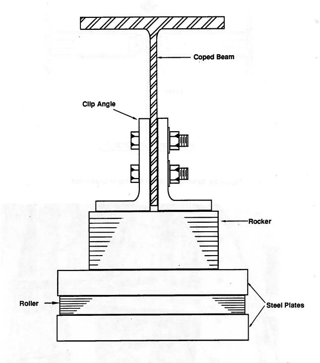
Figure 2.5 Clip Angle Connection at Cope End
