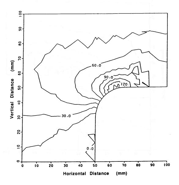
Figure 4.6 Stress Contour for 20 mm Cope Radius
