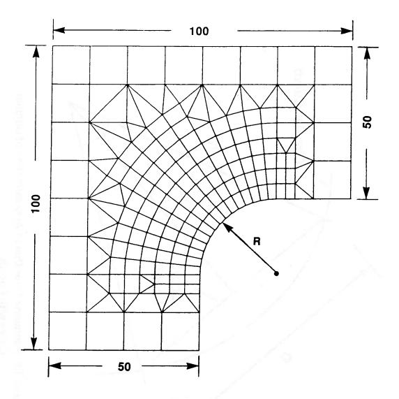
Figure 4.3 Typical Fine Mesh for Finite Element Analysis
