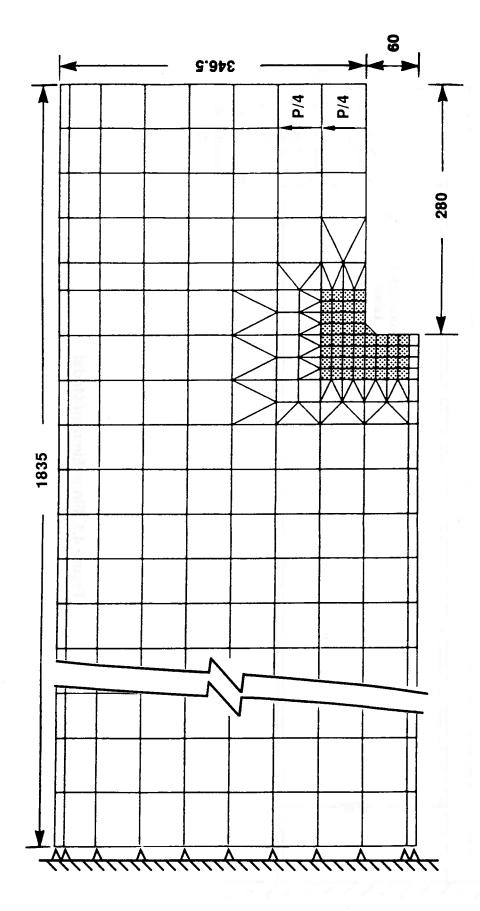
Typical Coarse Mesh for Finite Element Analysis Figure 4.2
