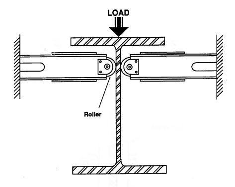
Figure 2.6 Schematic Lateral Bracing at Load Point
