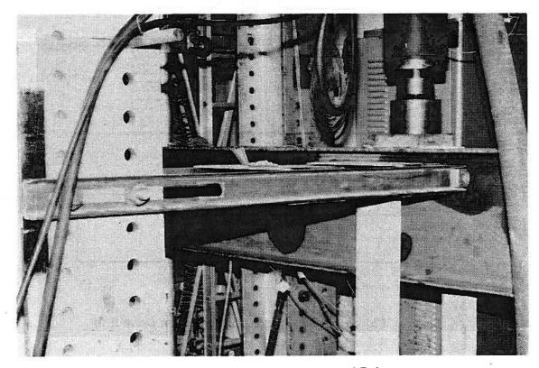
Figure 2.7 Lateral Bracing at Load Point
