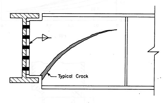
Figure 1.3 Typical Failed Coped Beam for FCCU Structural Failure
